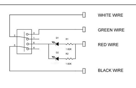
SCHEMATIC CIRCUIT 1A WITH LEDs
