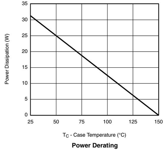
\* The power dissipation P<sub>D</sub> is based on T<sub>J(max.)</sub> = 150 °C, using junction-to-case thermal resistance, and is more useful in settling the upper dissipation limit for cases where additional heatsinking is used. It is used to determine the current rating, when this rating falls below the package limit.
