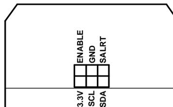
FIGURE 2. PIN CONFIGURATION DIAGRAM
