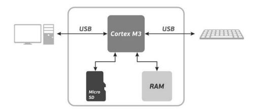
Pastilda has two USB ports: one for your keyboard, one to connect to your PC. Your OS will recognize Pastilda as a USB keyboard and a USB flash drive.
