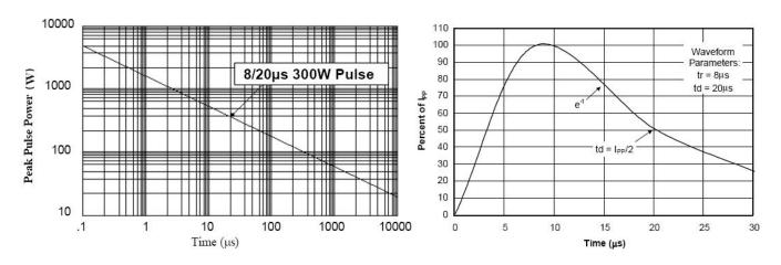
Figure 1. Peak Pulse Power Vs Pulse Time (µs)
