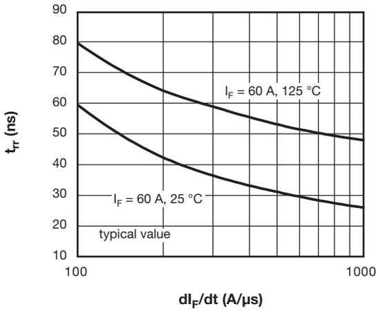
Fig. 7 - Typical Reverse Recovery vs.  $di_F/dt$
