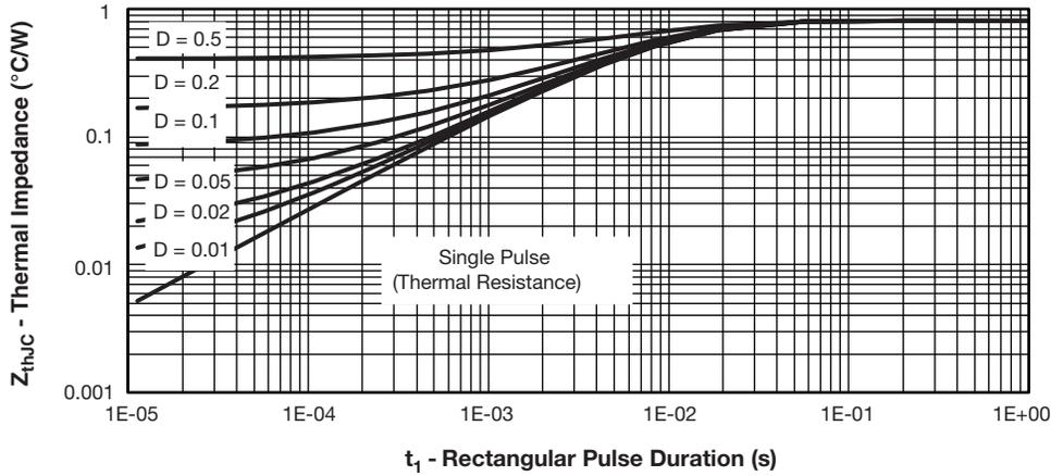
Fig. 4 - Maximum Thermal Impedance  $Z_{thJC}$  Characteristics
