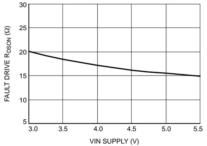
Figure 10. FAULT Drive R<sub>DS(on)</sub> vs. VIN Supply
