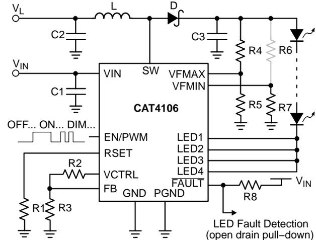
**Figure 27. Application Circuit for One LED String**
