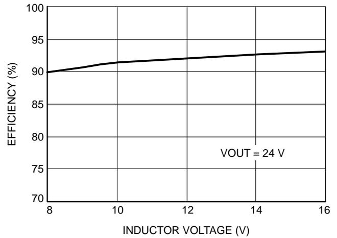
Figure 22. Efficiency vs. VL (VIN = 5 V)
