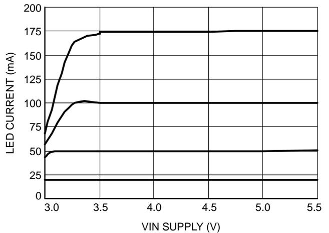
Figure 8. LED Channel Current vs. VIN Supply
