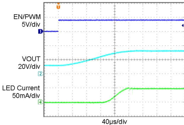
Figure 19. Power-Up 4 x 10 LEDs, 50 mA per Channel
