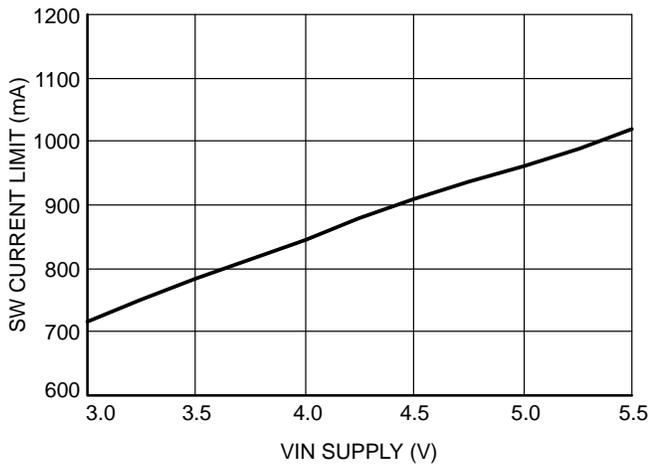
Figure 13. Switching Current Limit vs. VIN Supply
