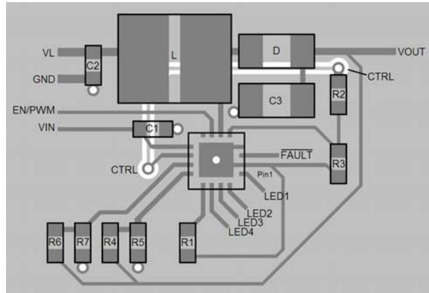
Figure 29. Recommended Layout for TQFN-16
