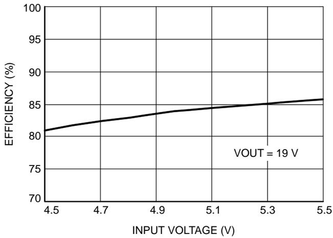
Figure 21. Efficiency vs. VIN (VIN = VL)
