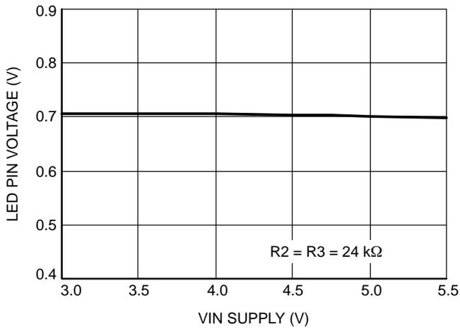
Figure 9. LED Channel Voltage vs. VIN Supply
