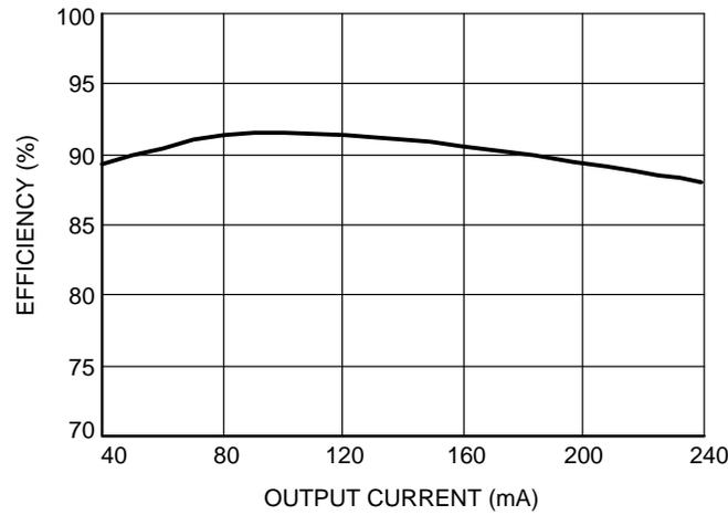
Figure 23. Efficiency vs. Output Current (9-LED String)
