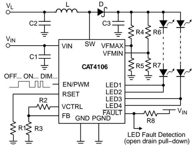
**Figure 28. Application Circuit for Two LED Strings**
