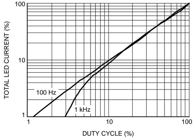
Figure 16. PWM Duty Cycle vs. LED Current
