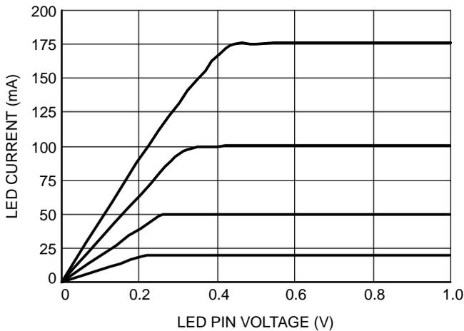
Figure 7. LED Channel Current vs. LED Pin Voltage
