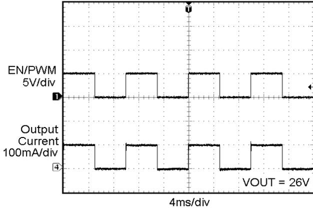
Figure 17. PWM Dimming 100 Hz
