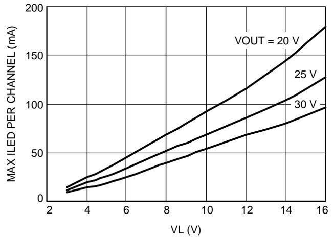
Figure 20. Maximum LED Current vs. VL Supply
