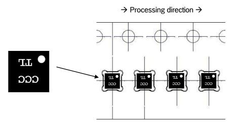
Figure 28: Orientation of the BMA222 devices relative to the tape
