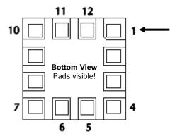
Figure 19 Pin-out bottom view
