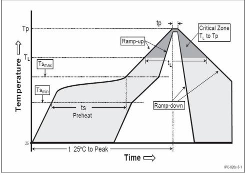
Figure 26: Soldering profile
