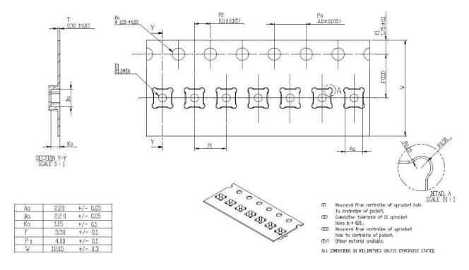
Figure 27: Tape and reel dimensions in mm
