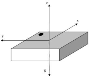
Figure 24: Orientation of sensing axis
