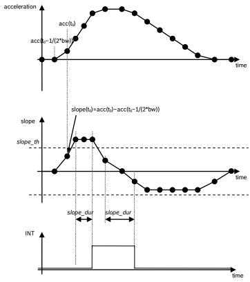
Figure 6: Principle of any-motion detection
