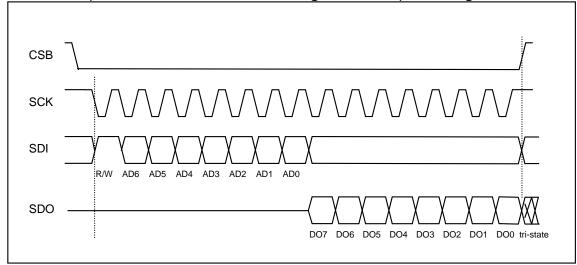
Figure 12: 4-wire basic SPI read sequence (mode '11')
