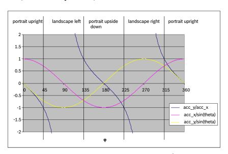
Figure 9: Typical orientation switching conditions w/o hysteresis
