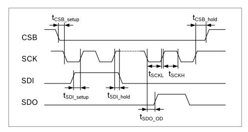
Figure 10: SPI timing diagram
