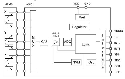
Figure 1: Block diagram of BMA222
