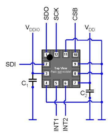
Figure 20: 4-wire SPI connection
