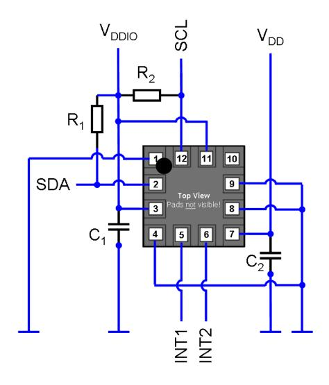
Figure 22: I<sup>2</sup>C connection
