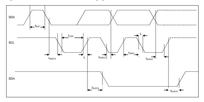
Figure 15: I<sup>2</sup>C timing diagram
