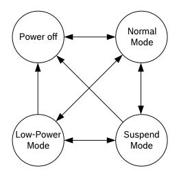
Figure 3: Power mode transition diagram
