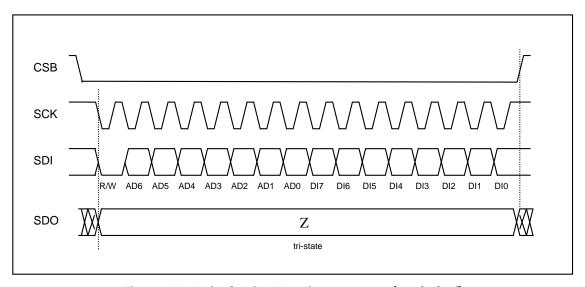
Figure 11: 4-wire basic SPI write sequence (mode '11')
