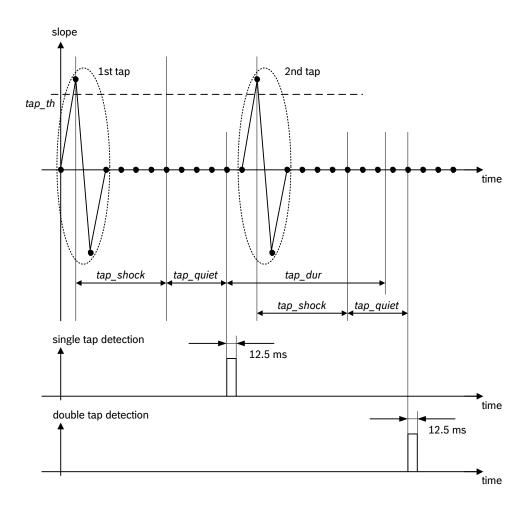
Figure 7: Timing of tap detection
