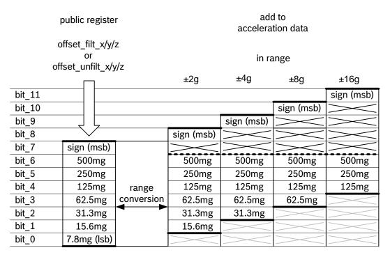
Figure 4: Principle of offset compensation
