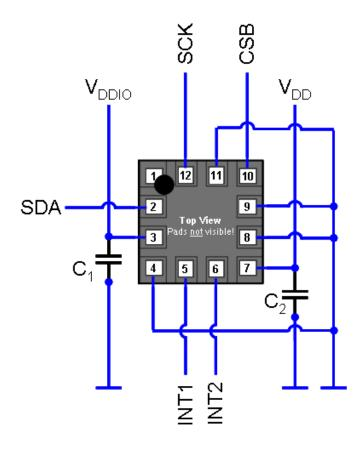
Figure 21: 3-wire SPI connection
