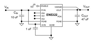
Figure 1. Typical Application Circuit
