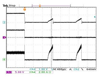
Output Over Load at 2 A Load ( $V_{IN} = 5 V$ ,  $V_{OUT} = 1.2 V$ ) CH2: VOUT, CH3: POK, CH4: INDUCTOR
