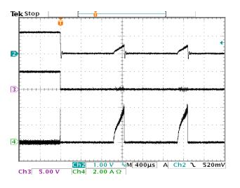
Output Over Load at No Load (VIN = 5 V, VOUT = 1.2 V) CH2: VOUT, CH3: POK, CH4: INDUCTOR
