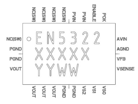
Figure 2. Pin Diagram, Top View.
