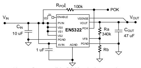
\* Leave R<sub>POK</sub> open if the POK function is not used. **Figure 6. Typical Application Circuit with External Resistor Divider.** (*NOTE:* Enable can be separated from PVIN if the application requires it)
