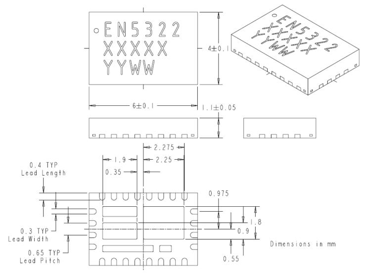
Figure 9. EN5322QI Package Dimensions
