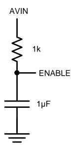
Figure 5: ENABLE Delay Circuit
