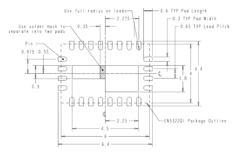
Figure 8. Recommended Footprint for PCB.
