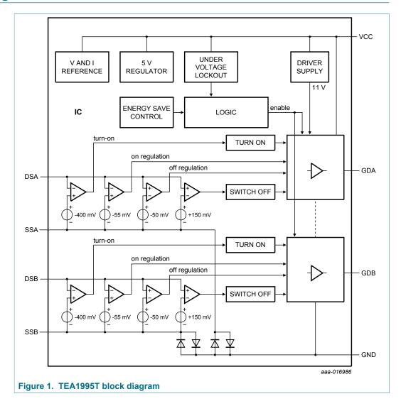
GreenChip dual synchronous rectifier controller
