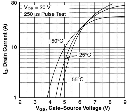
Figure 2. Transfer Characteristics
