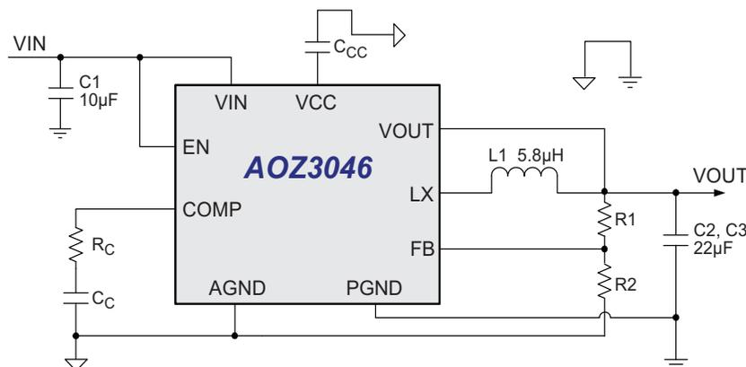
Figure 1. 5 V, 4 A Synchronous Buck Regulator,  $F_s = 500$  KHz
