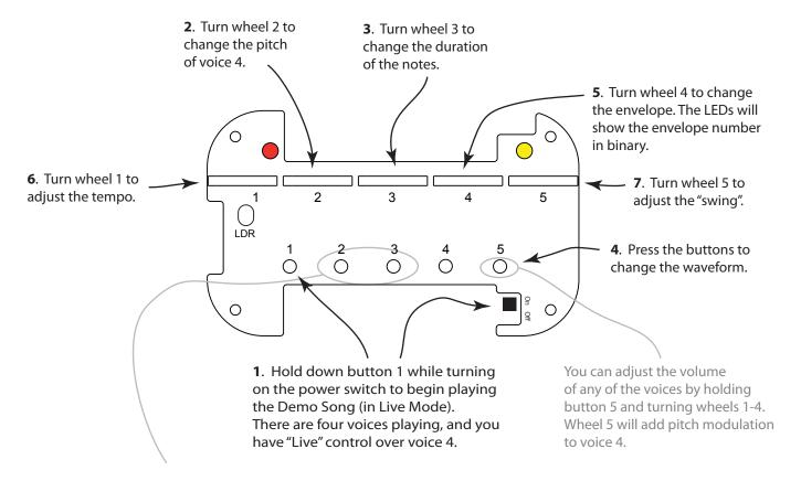
Press buttons 2 and 3 to transfer pitch control to the photocell (LDR). Try not to block the photocell while you do this, because it will be calibrated to the ambient light level. Now you can move your hand over the photocell or open and close the lid to change the pitch of voice 4. To recalibrate the photocell to a different light level you can press buttons 2 and 3 again. If you turn wheel 2 it will take pitch control back from the photocell.
