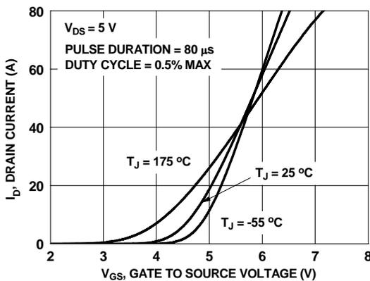
Figure 5. Transfer Characteristics
