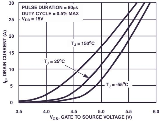
**Figure 7. Transfer Characteristics**
