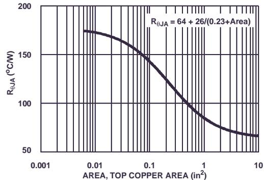
Figure 21. Thermal Resistance vs Mounting Pad Area
