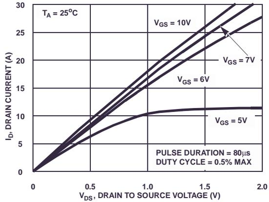
**Figure 8. Saturation Characteristics**
