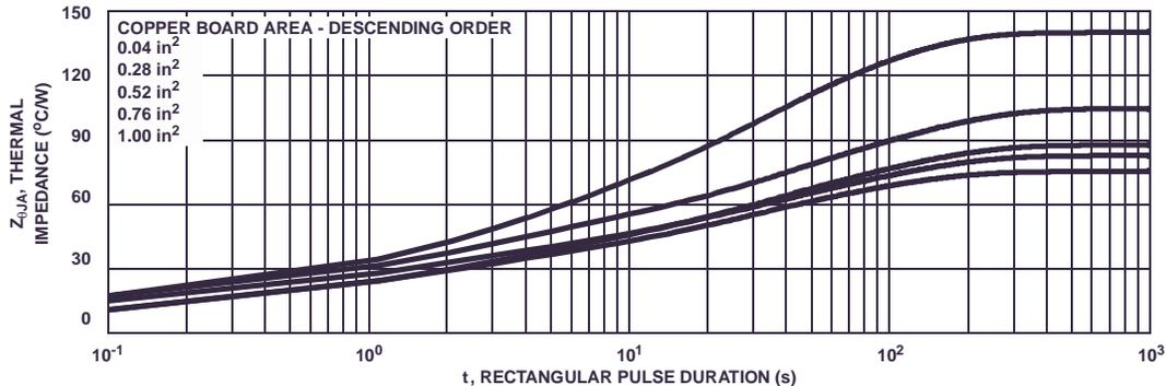
Figure 22. Thermal Impedance vs Mounting Pad Area
