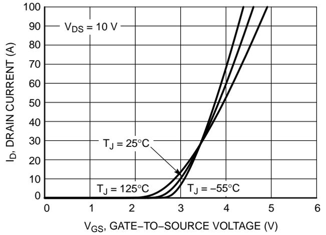
Figure 2. Transfer Characteristics
