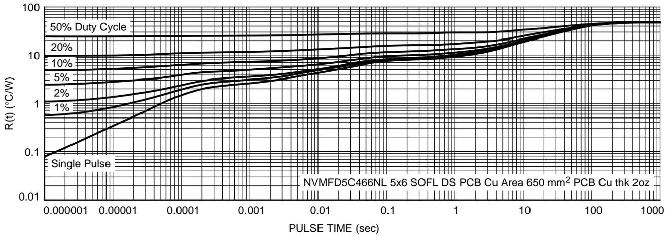
Figure 13. Thermal Characteristics
