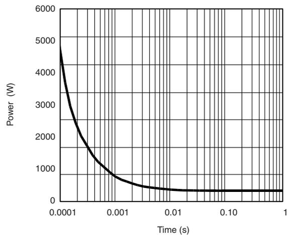
Single Pulse Power, Junction-to-Case ( $T_C = 25\text{ }^\circ\text{C}$ )
