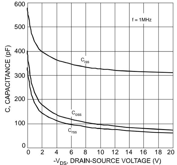
Fig. 6: Typical Capacitance
