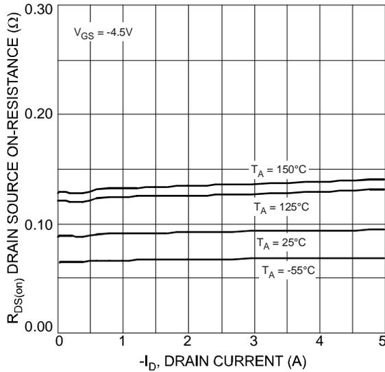
Fig. 5 Drain-Source On-Resistance Vs. Drain Current and Temperature
