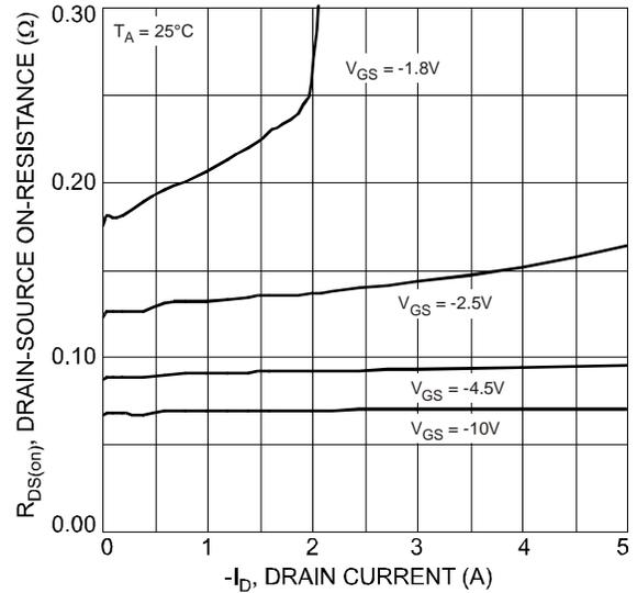
Fig. 4 On-Resistance vs Drain Current and Gate Voltage
