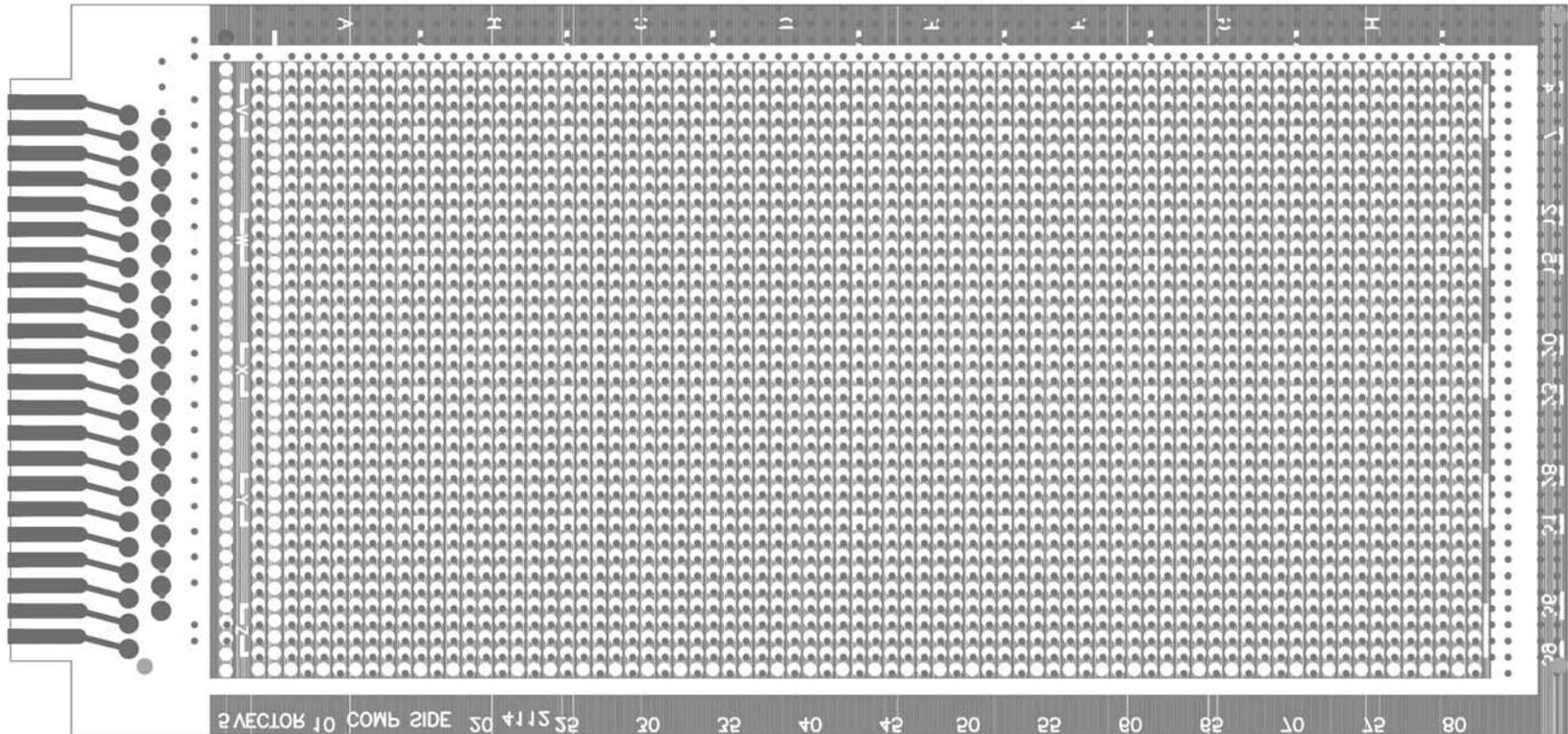
5. In accordance with consumer protection policies, we suggest you inspect the board before assembly to verify adequate clearance will exist between the ground plane surrounding the holes and any leads or terminals installed in holes so that shorting will not occur. Terminals inserted into the holes in the ground plane areas, and closely spaced contact finger areas may cause short circuits unless:
