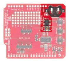
The Real-Time Clock is used to keep accurate time, which is often useful in security protocols. The clock on the CryptoShield is the DS3231M. It's attached to the I2C bus with an address of  $0\times68$ .
