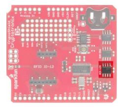
The Atmel AES132 is an AES encrypted EEPROM that can store up to 32Kb of data. Specifically, it uses AES with a 128 bit key in CCM mode.
