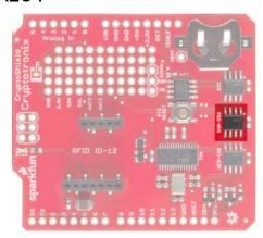
The Atmel ATSHA204 is an authentication chip that performs SHA-256 and HMAC-256. It can store up to 16 secret keys that can be used for shared-secret authentication between two devices with an ATSHA204 or between a ATSHA204 and a remote server. It also can produce random numbers with its on-chip random number generator. The ATSHA204 on the CryptoCape is the I2C version of our Breakout Board version. It's also on the Electric Imp.
