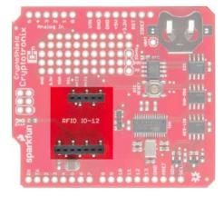
The RFID socket on the shield works best with SparkFun's RFID ID-12LA. Simply attach the reader and when a tag is read, the reader will write out to the Arduino hardware serial lines. It will also flash the "stat" light on the CryptoShield. Using the ID-12LA, the RFID tag, button, and capsule can all be read.
