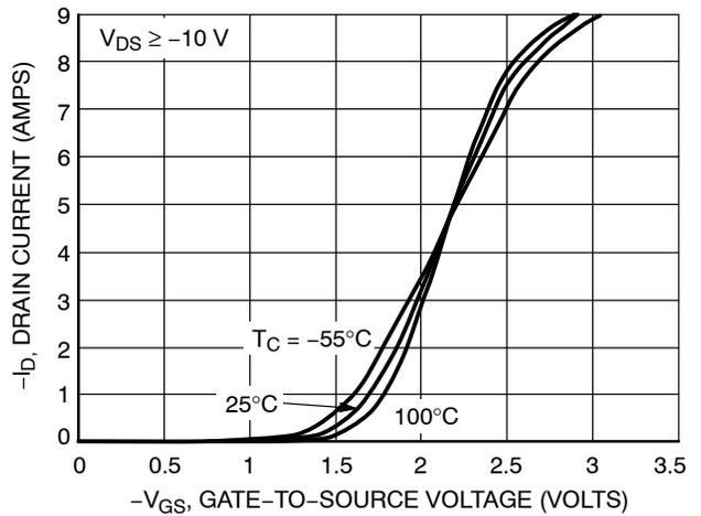
Figure 2. Transfer Characteristics
