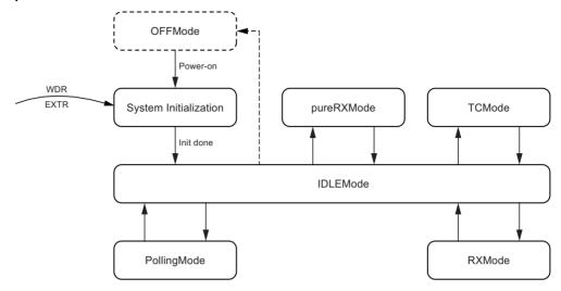
After connecting the supply voltage to the VS pin, the Atmel ATA5780N always starts in OFFMode. All internal circuits are disconnected from the power supply. Therefore, no SPI communication is supported. The Atmel ATA5780N can be woken up by activating the PWRON pin or one of the NPWRONx pins. This triggers the power-on sequence. After firmware initialization the Atmel ATA5780N reaches the IDLEMode.
