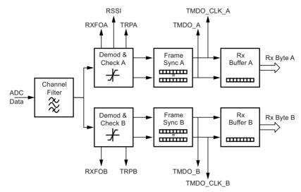
The channel filter determines the receiver bandwidth. Its output is used for both receiving paths A and B. Therefore, it has to be configured to be suitable for both. The receiving paths A and B are identical and consist of an ASK/FSK demodulator with attached signal checks, a frame synchronizer supporting pattern based search for the telegram start and a 1 byte hardware buffer for received data.
