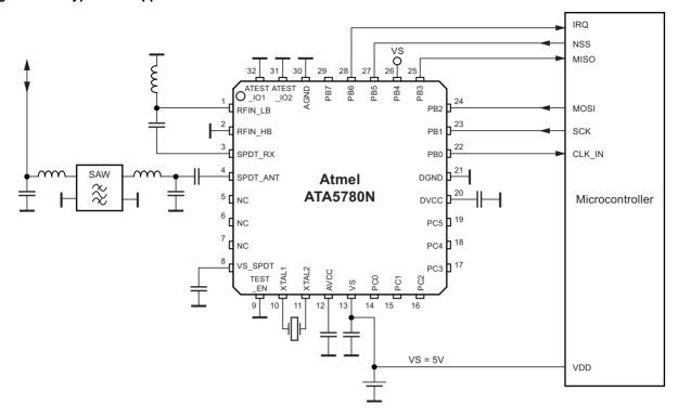
Figure 1-2 shows the typical application circuit with an external host microcontroller running from a 5V supply. For a 3V application VS and VS SDPT have to be shorted. The pin PB4 (PWRON) is directly connected to VS and the Atmel® ATA5780N enters the IDLEMode after power-on. The Atmel ATA5780N can work autonomously while the microcontroller stays powered down to achieve low current consumption while being sensitive to RF telegrams.
