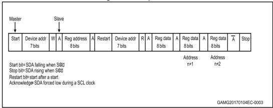
Figure 6: Write operation
