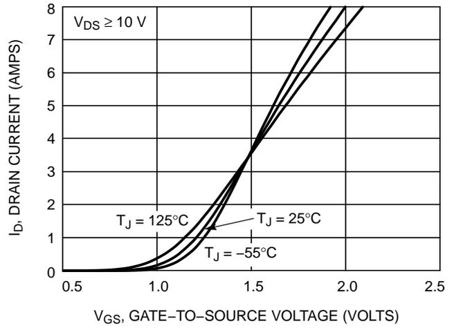
Figure 2. Transfer Characteristics
