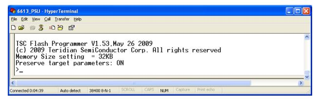
Type the "H" command at the > prompt on the terminal and select Transfer -> Send Text File (as shown below). Do not select Send File. This .hex file must have previously been processed with the CHKSUM.exe utility.
