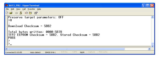
5. To program the device's flash using the flash image that was just programmed in the TFP2's EEPROM in steps 3 and 4 above, type the "P" command at the > prompt or simply push the Program button on the TFP2. If the programming is successful, a "PASS" message will be displayed. The Firmware programming is now complete.
