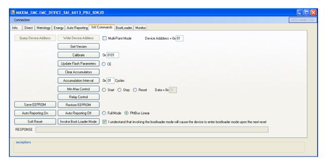
2. Power cycle the device. It will enter the Boot Load mode. This can be verified by observing the DIO4 pin, which produces 15 ms pulses when the boot loader is in operation.
