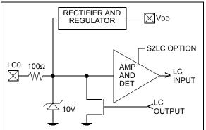
FIGURE 2-4: DATA PIN DIAGRAM
