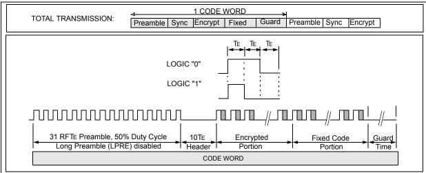
FIGURE 3-5: PWM TRANSMISSION FORMAT—MOD = 0
