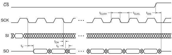
Figure 15-3.  $\overline{\text{WP}}$  Timing for Write Status Register Command When SPRL = 1
