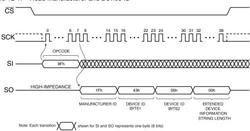
Figure 12-1. Read Manufacturer and Device ID
