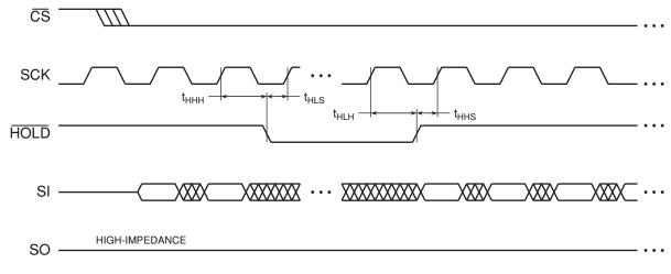
Figure 15-5. HOLD Timing – Serial Output
