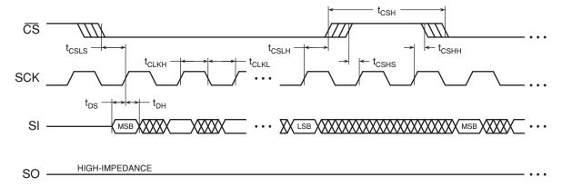
Figure 15-2. Serial Output Timing
