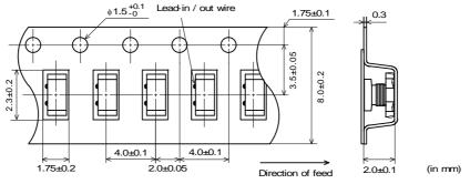
•Dimension of the Cavity is measured at the bottom side.
