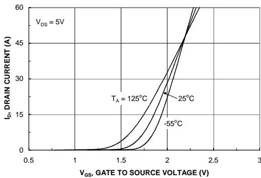
Figure 5. Transfer Characteristics.
