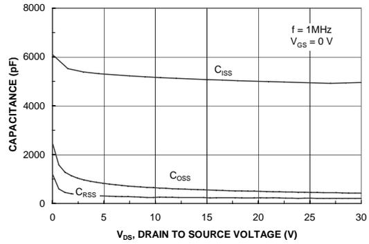
Figure 8. Capacitance Characteristics.
