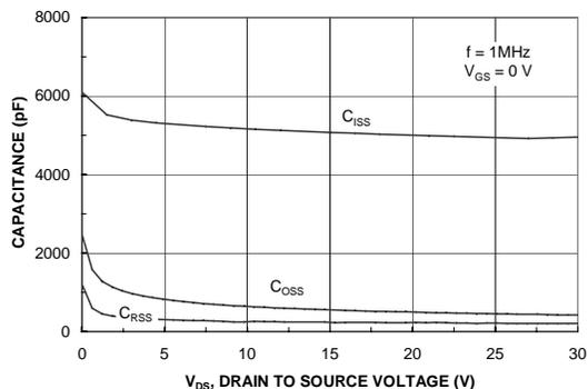
Figure 8. Capacitance Characteristics.
