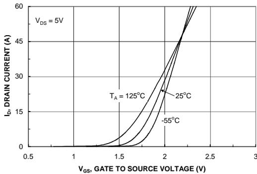
Figure 5. Transfer Characteristics.
