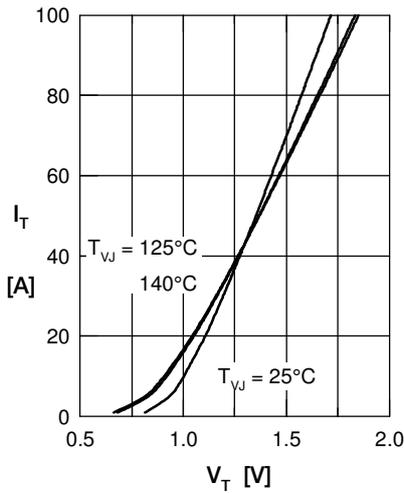
Fig. 1 Forward characteristics
