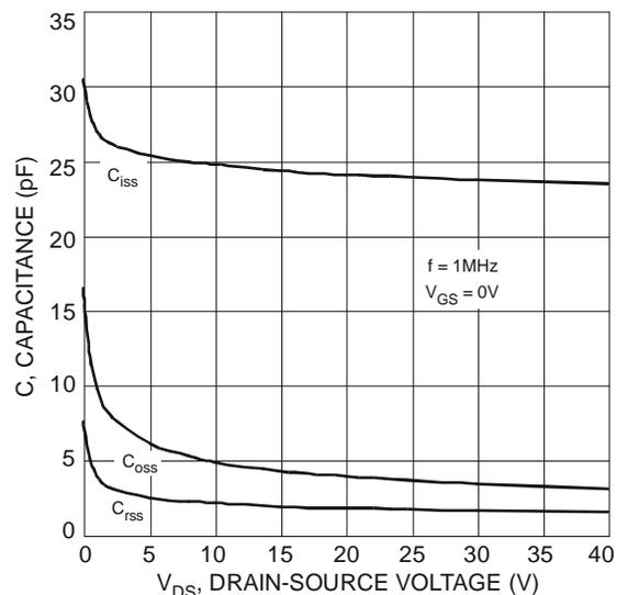
Fig. 6 Typical Capacitance
