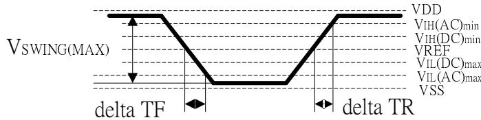
$$\text{Falling Slew} = \frac{V_{REF}-V_{IL(AC)}_{max}}{\text{delta TF}} \quad \text{Rising Slew} = \frac{V_{IH(AC)}_{min}-V_{REF}}{\text{delta TR}}$$
