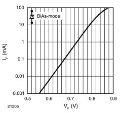
Figure 4. Typical Forward Current I<sub>F</sub> vs. Forward Voltage V<sub>F</sub>
