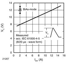
Figure 6. Typical Peak Clamping Voltage V\_C vs. Peak Pulse Current  $\rm I_{PP}$
