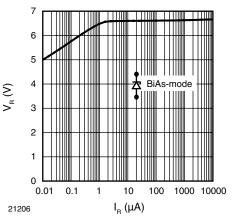
Figure 5. Typical Reverse Voltage  $\rm V_R$  vs. Reverse Current  $\rm I_R$
