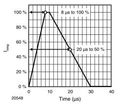
Figure 2. 8/20 µs Peak Pulse Current Wave Form (acc. IEC 61000-4-5)
