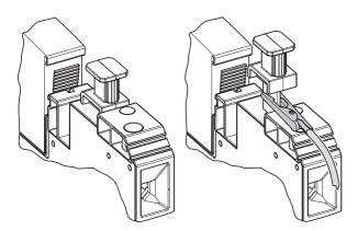
Figure 7 Test equipment field connection
