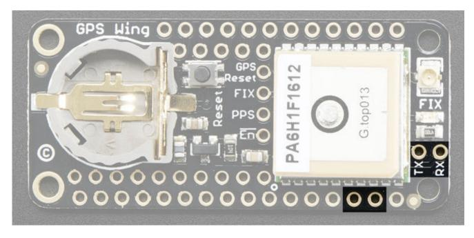
The GPS module, like pretty much all GPS's, communicates over UART serial. It sends ASCII NMEA setences from the GPS TX pin to the microcontroller RX pin and can be controlled to change its data output from the GPS RX pin. Logic level is 3.3V for both.
