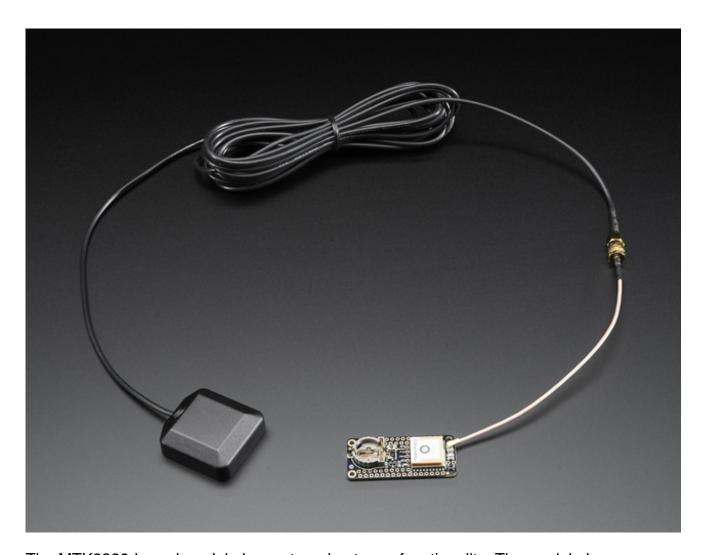
The MTK3339-based module has external antenna functionality. The module has a standard ceramic patch antenna that gives it -165 dB sensitivity, but when you want to have a bigger antenna, you can snap on any 3V active GPS antenna via the uFL connector. The module will automatically detect the active antenna and switch over! Most GPS antennas use SMA connectors so you may want to pick up one of our uFL to SMA adapters. (http://adafru.it/851)
