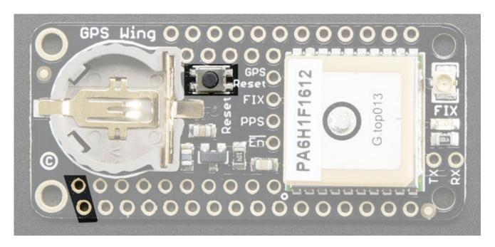
There is a small button that will connect the *microcontroller* RESET pin to ground for resetting it. Handy to restart the Feather. Note that this is not connected to GPS reset unless you short the jumper on the back!
