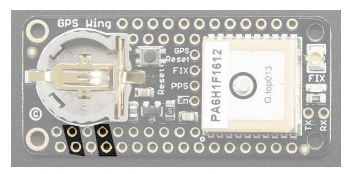
The GPS module runs from +3.3V power and uses 3V logic. the GPS is powered directly from the **3V** and **GND** pins on the bottom left of the Feather. Each Feather has a regulator to provide clean 3V power from USB or battery power.
