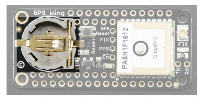
The GPS does not *require* but does benefit by having a coin cell backup battery. You can install any "CR1220" sized battery into the holder. The GPS will automatically detect the battery and use it as a backup for the ephemeris memory
