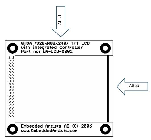
Figure 2 - 3.2 inch QVGA TFT Color LCD Board Optimum Viewing Angle
