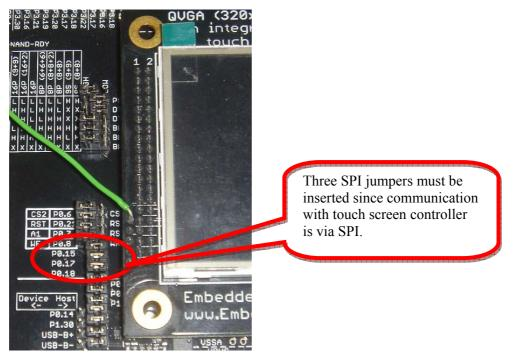
Figure 4 – Picture of Wire to Pin 45 on Display Module
