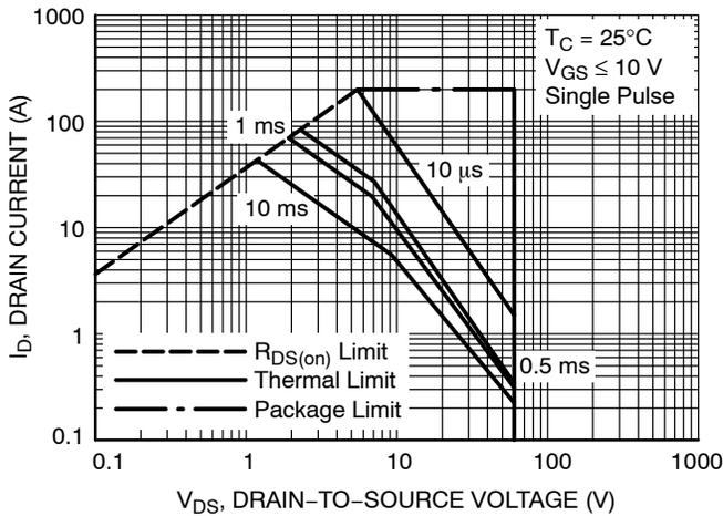
Figure 11. Maximum Rated Forward Biased Safe Operating Area
