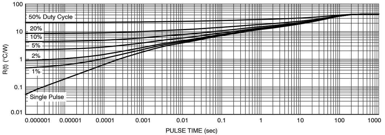
**Figure 13. Thermal Characteristics**
