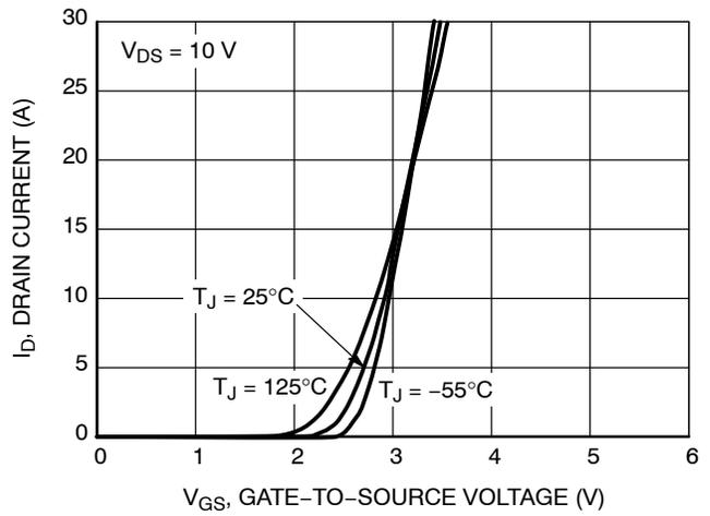
Figure 2. Transfer Characteristics
