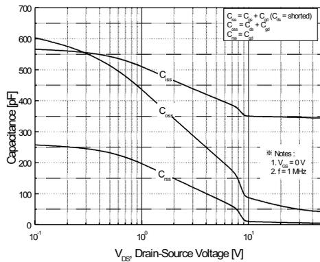
Figure 5. Capacitance Characteristics
