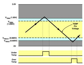
FIGURE 6. CRITICAL VOLTAGE LEVELS FOR TEMP PIN
