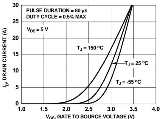
Figure 5. Transfer Characteristics
