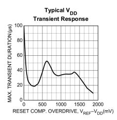
Figure 3. Typical VDD Transient Response
