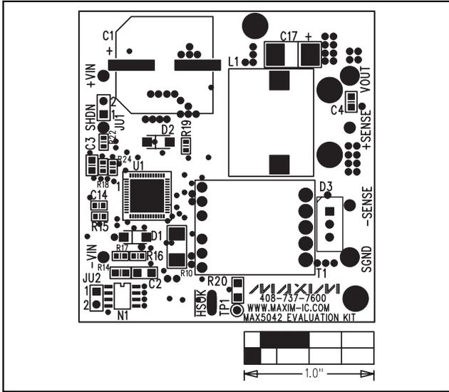
Figure 6. MAX5042 EV Kit Component Placement Guide—Component Side
