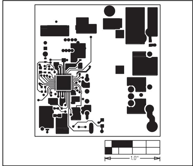
Figure 7. MAX5042 EV Kit PC Board Layout—Component Side
