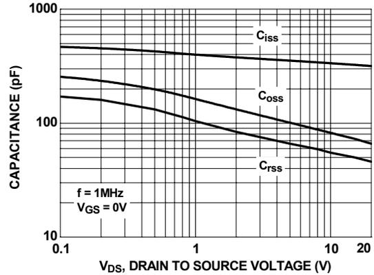
**Figure 8. Capacitance Characteristics**
