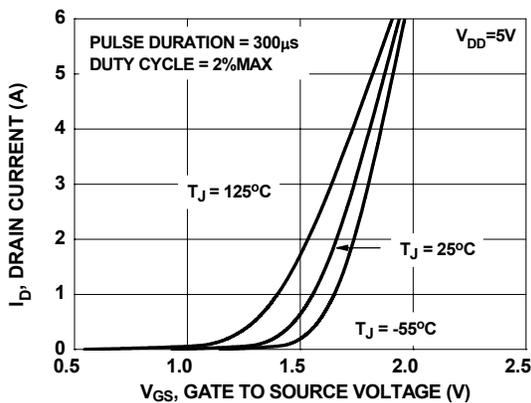
**Figure 5. Transfer Characteristics**
