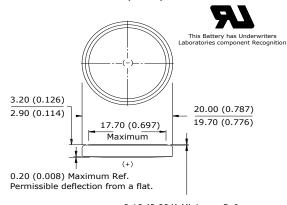
0.10 (0.004) Minimum Ref. (Applies to top edge of gasket or edge of crimp, whichever is higher.)
