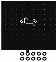
a. 42  $^{\circ}\text{C}/\text{W}$  when mounted on a 1 in<sup>2</sup> pad of 2 oz copper
