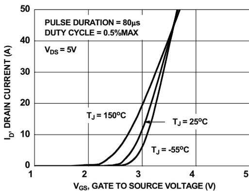
Figure 5. Transfer Characteristics
