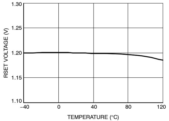
Figure 12. RSET Pin Voltage vs. Temperature
