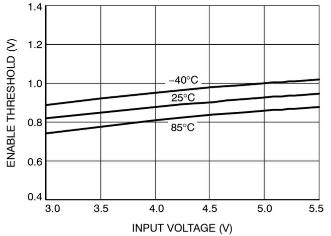
**Figure 15. EN/PWM Threshold vs. VIN**
