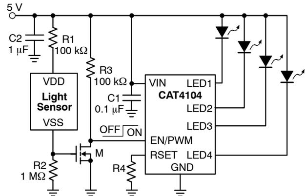
**Figure 22. Nightlight Detection**
