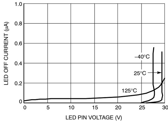
Figure 13. LED Off Current vs. LED Pin Voltage
