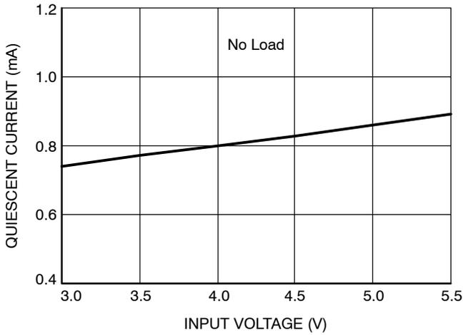
**Figure 3. Quiescent Current vs. Input Voltage (RSET Open)**
