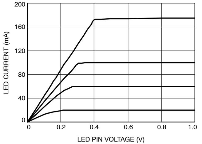
**Figure 6. LED Dropout vs. LED Pin Voltage**
