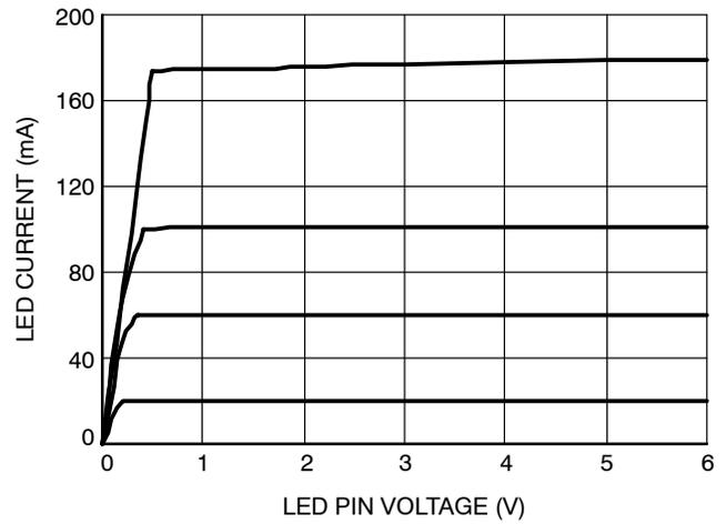
Figure 10. LED Current vs. LED Pin Voltage
