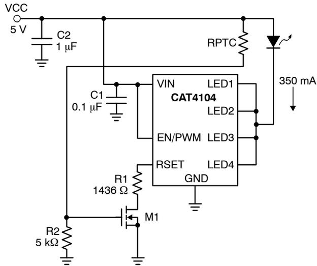
**Figure 23. LED Current Derating**
