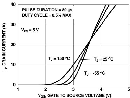
**Figure 5. Transfer Characteristics**
