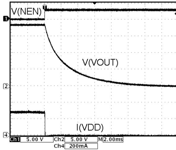
FIGURE 10. SHUT DOWN @ SEL = 1 ( $V_{DD} = 3.6V$ ,  $R_L = 360\Omega$ )
