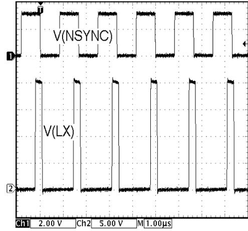
FIGURE 18. LX SYNCHRONIZATION WITH  $f(\text{SYNC}) = 600\text{kHz}$
