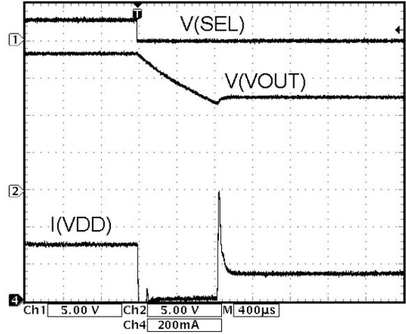
FIGURE 9. 18V->12V TRANSITION ( $V_{DD} = 3.6V$ ,  $R_L = 360\Omega$ )
