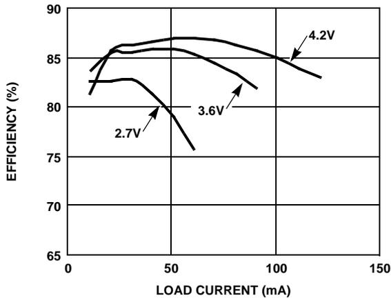
FIGURE 2. EFFICIENCY vs LOAD CURRENT ( $V_{OUT} = 18.3V$ )
