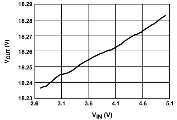
FIGURE 12. LINE REGULATION (I<sub>OUT</sub> = 30mA)
