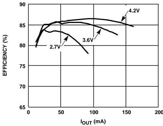
FIGURE 4. EFFICIENCY vs  $I_{OUT}$  ( $V_{OUT} = 12.6V$ )
