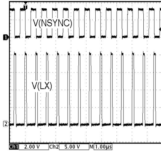
FIGURE 19. LX SYNCHRONIZATION WITH  $f(\text{SYNC}) = 1.4\text{MHz}$
