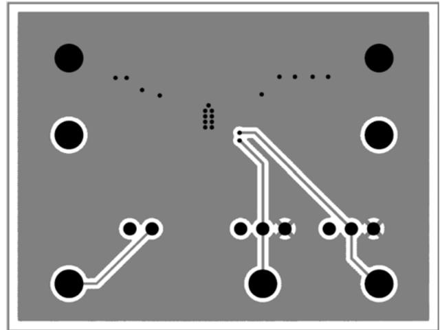
FIGURE 22. BOTTOM LAYER of the DEMO BOARD
