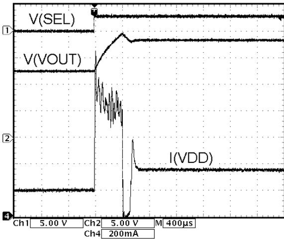
FIGURE 8. 12V->18V TRANSITION ( $V_{DD} = 3.6V$ ,  $R_L = 360\Omega$ )
