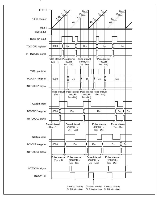
When executing pulse width measurement in the free-running timer mode, four pulse widths can be measured with one channel.
