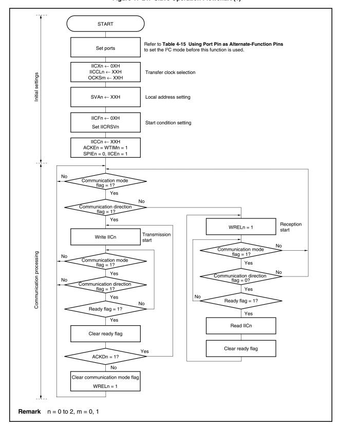
Figure 17-21. Slave Operation Flowchart (1)
