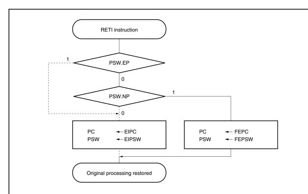
Caution When the EP and NP bits are changed by the LDSR instruction during non-maskable interrupt servicing, in order to restore the PC and PSW correctly during recovery by the RETI instruction, it is necessary to set the EP bit back to 0 and the NP bit back to 1 using the LDSR instruction immediately before the RETI instruction.
