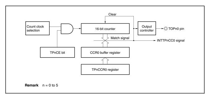
Figure 7-2. Configuration of Interval Timer
