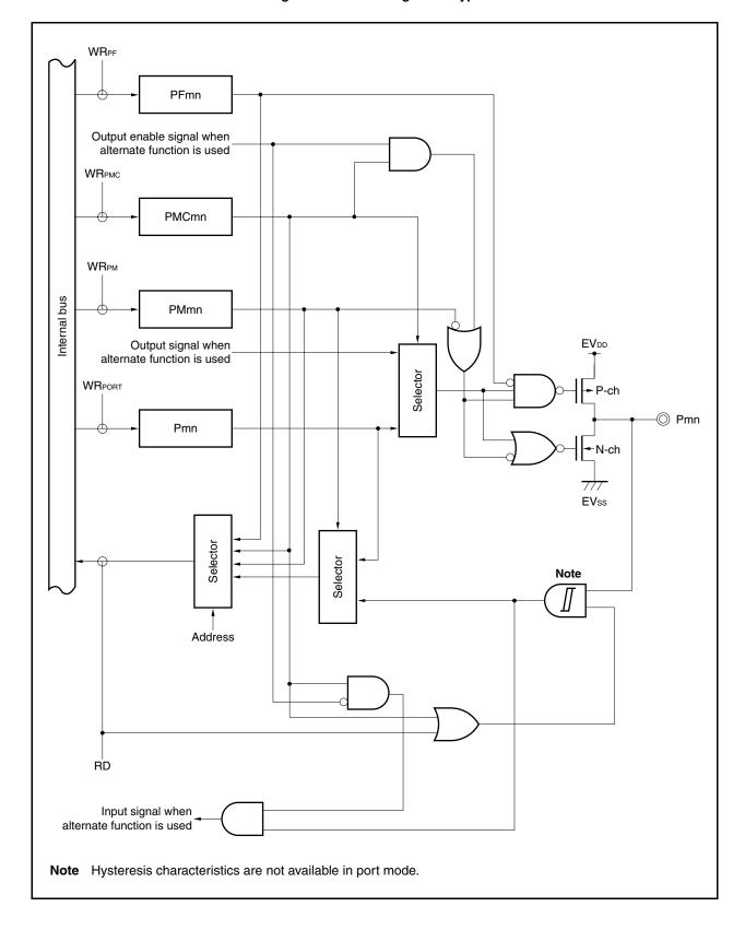
Figure 4-9. Block Diagram of Type E-3
