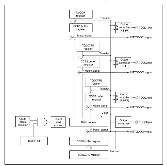
Figure 8-24. Configuration in PWM Output Mode
