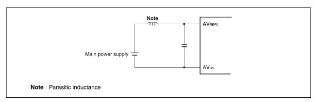
Figure 13-15. AVREFO Pin Processing Example
