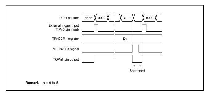
If the trigger is detected immediately before the INTTPnCC1 signal is generated, the INTTPnCC1 signal is not generated, and the 16-bit counter is cleared to 0000H and continues counting. The output signal of the TOPn1 pin remains active. Consequently, the active period of the PWM waveform is extended.
