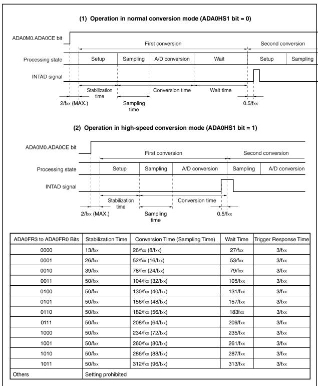
**Remark** The above timings are when a trigger generates within the stabilization time. If the trigger generates after the stabilization time, a trigger response time is inserted.
