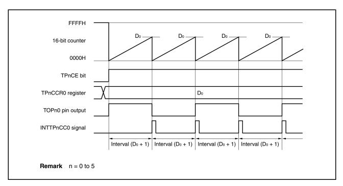
When the TPnCE bit is set to 1, the value of the 16-bit counter is cleared from FFFFH to 0000H in synchronization with the count clock, and the counter starts counting. At this time, the output of the TOPn0 pin is inverted. Additionally, the set value of the TPnCCR0 register is transferred to the CCR0 buffer register.
