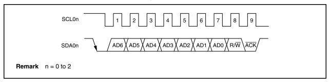
When the local address is received,  $\overline{ACK}$  is automatically generated regardless of the value of the ACKEn bit. No  $\overline{ACK}$  is generated if the received address is not a local address (NACK).
