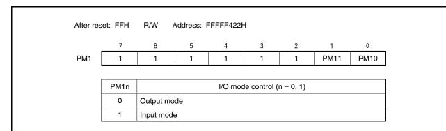
Cautions 1. When using P1n as the alternate function (ANOn pin output), set the PM1n bit to 1.
