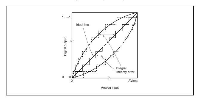
Figure 13-21. Integral Linearity Error
