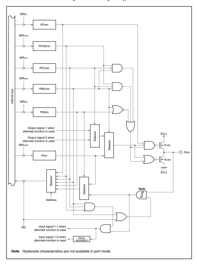
Figure 4-21. Block Diagram of Type U-5
