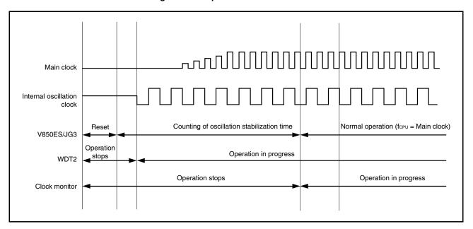
Figure 22-5. Operation After Reset Release
