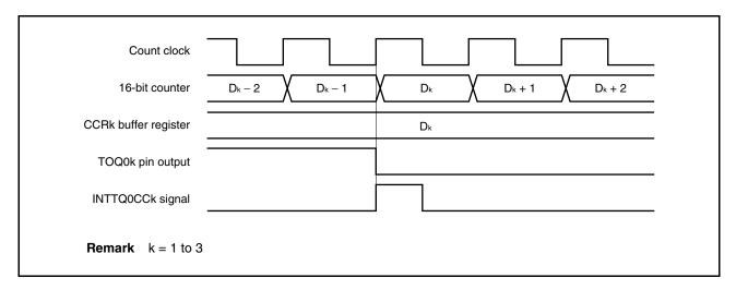
Usually, the INTTQ0CCk signal is generated in synchronization with the next counting up after the count value of the 16-bit counter matches the value of the TQ0CCRk register.
