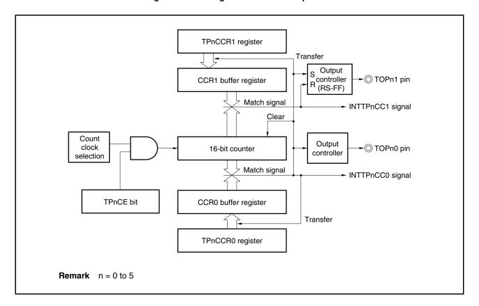
Figure 7-24. Configuration in PWM Output Mode
