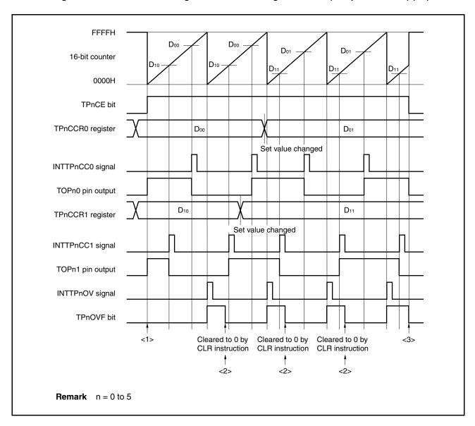
Figure 7-32. Software Processing Flow in Free-Running Timer Mode (Compare Function) (2/2)
