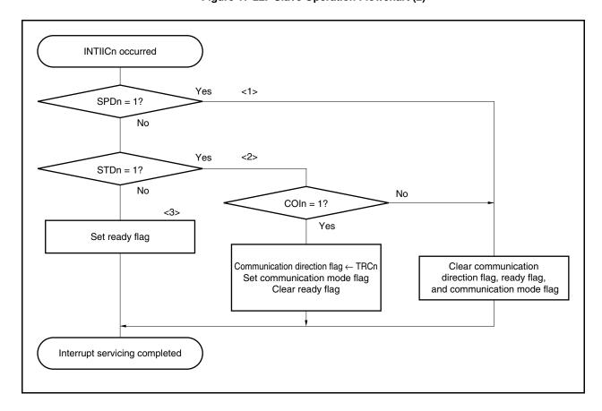
Figure 17-22. Slave Operation Flowchart (2)
