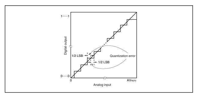
Figure 13-17. Quantization Error
