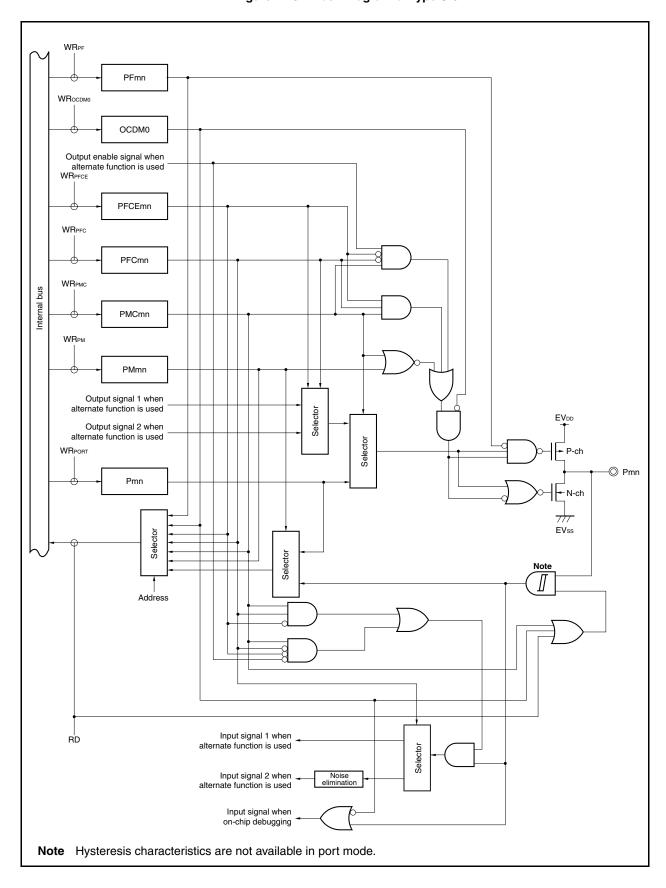
Figure 4-25. Block Diagram of Type U-9
