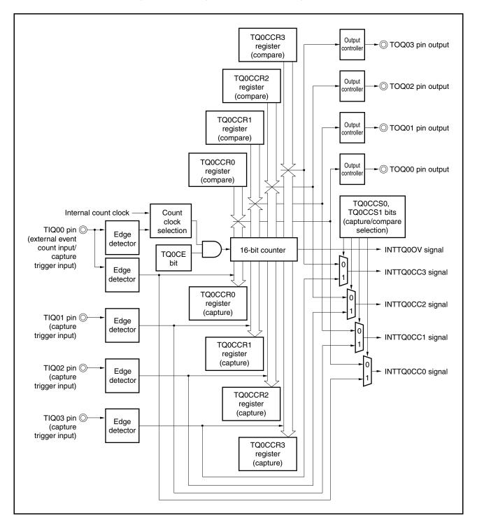
When the TQ0CE bit is set to 1, 16-bit timer/event counter Q starts counting, and the output signals of the TQ000 to TQQ03 pins are inverted. When the count value of the 16-bit counter later matches the set value of the TQ0CCRm register, a compare match interrupt request signal (INTTQ0CCm) is generated, and the output signal of the TQQ0m pin is inverted.
