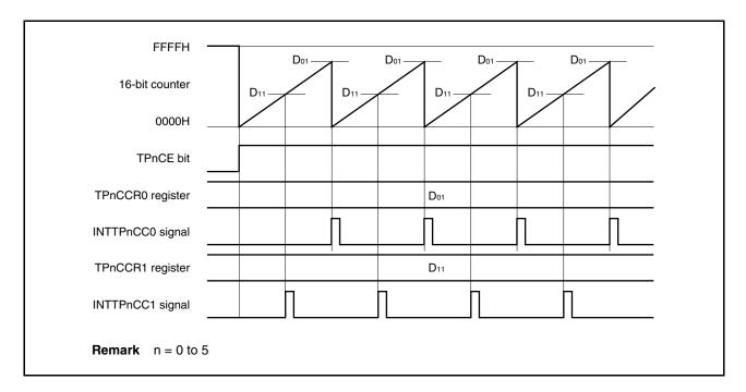
Figure 7-14. Timing Chart When D<sub>01</sub> ≥ D<sub>11</sub>
