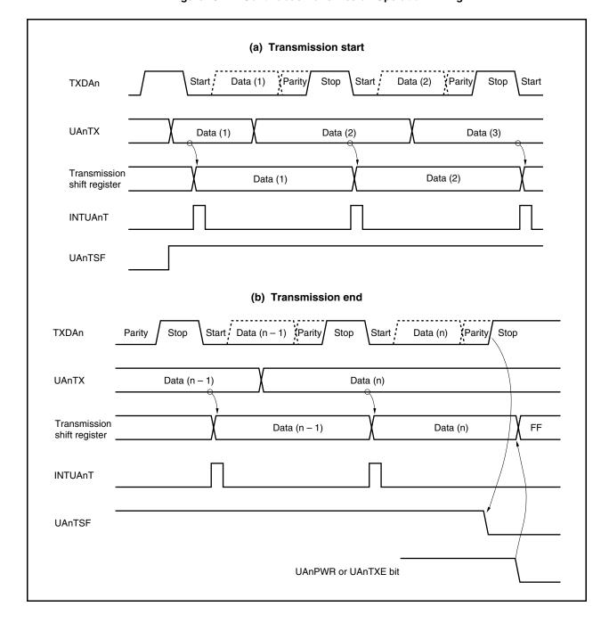
Figure 15-12. Continuous Transmission Operation Timing
