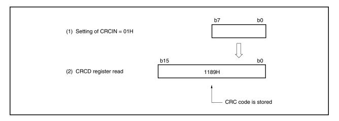
The code when 01H is sent LSB first is (1000 0000). Therefore, the CRC code from generation polynomial  $X^{16} + X^{12} + X^6 + 1$  becomes the remainder when (1000 0000)  $X^{16}$  is divided by (1 0001 0000 0010 0001) using the modulo-2 operation formula.
