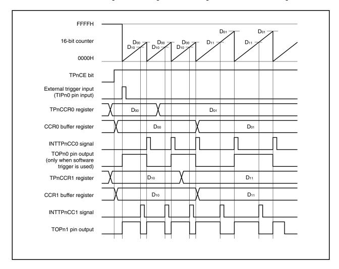
In order to transfer data from the TPnCCRm register to the CCRm buffer register, the TPnCCR1 register must be written.
