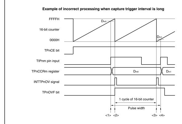
The following problem may occur when long pulse width is measured in the free-running timer mode.
