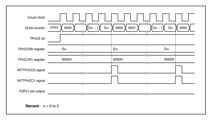
To output a 100% waveform, set a value of (set value of TPnCCR0 register + 1) to the TPnCCR1 register. If the set value of the TPnCCR0 register is FFFFH, 100% output cannot be produced.
