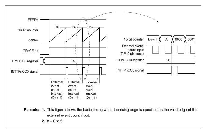
When the TPnCE bit is set to 1, the value of the 16-bit counter is cleared from FFFFH to 0000H. The counter counts each time the valid edge of external event count input is detected. Additionally, the set value of the TPnCCR0 register is transferred to the CCR0 buffer register.
