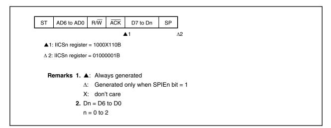
(6) When arbitration loss occurs due to low level of SDA0n pin when attempting to generate a restart condition
