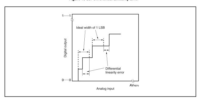
Figure 13-20. Differential Linearity Error
