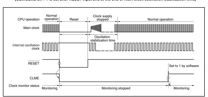
Figure 23-3. Clock Monitor Status After RESET Input
