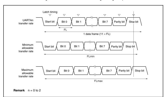
Figure 15-17. Allowable Baud Rate Range During Reception
