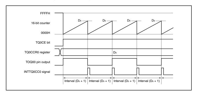
When the TQ0CE bit is set to 1, the value of the 16-bit counter is cleared from FFFFH to 0000H in synchronization with the count clock, and the counter starts counting. At this time, the output of the TQ000 pin is inverted. Additionally, the set value of the TQ0CCR0 register is transferred to the CCR0 buffer register.
