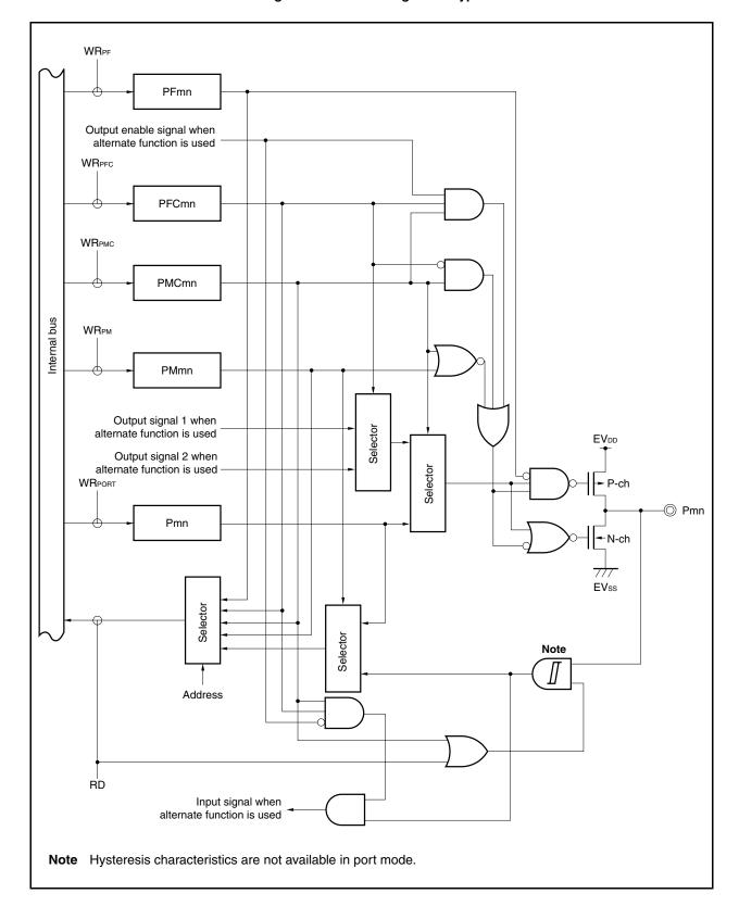
Figure 4-13. Block Diagram of Type G-5
