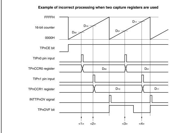
The following problem may occur when two pulse widths are measured in the free-running timer mode.
