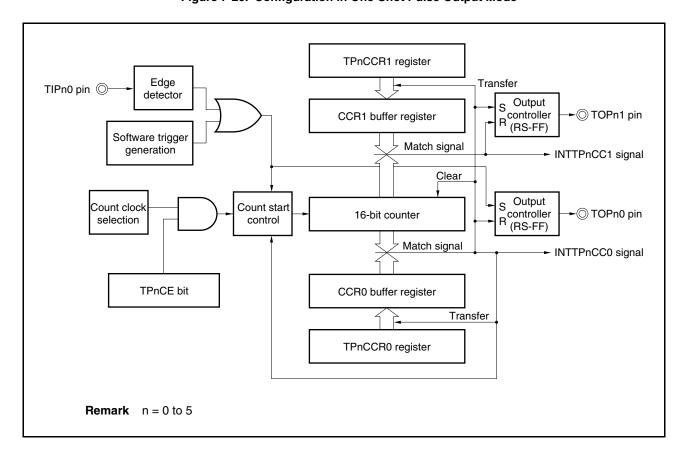
Figure 7-20. Configuration in One-Shot Pulse Output Mode
