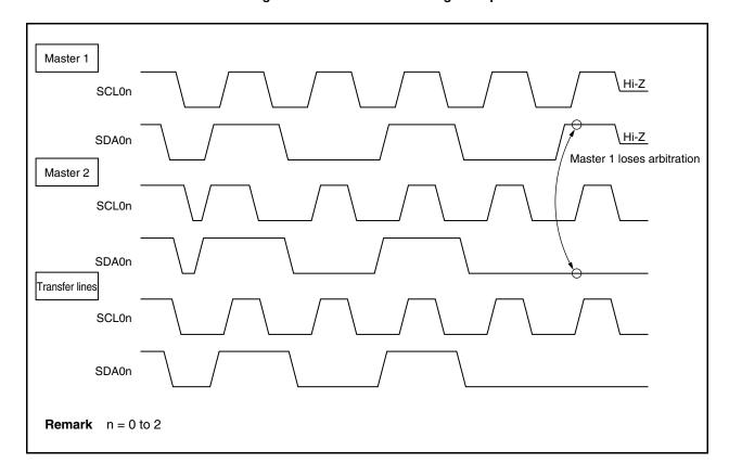
Figure 17-14. Arbitration Timing Example
