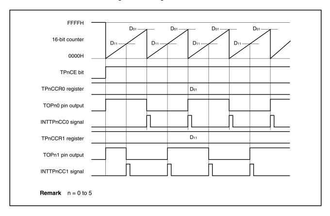
If the set value of the TPnCCR1 register is greater than the set value of the TPnCCR0 register, the count value of the 16-bit counter does not match the value of the TPnCCR1 register. Consequently, the INTTPnCC1 signal is not generated, nor is the output of the TOPn1 pin changed.
