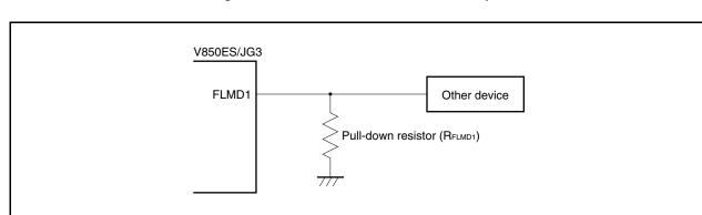
Figure 27-11. FLMD1 Pin Connection Example
