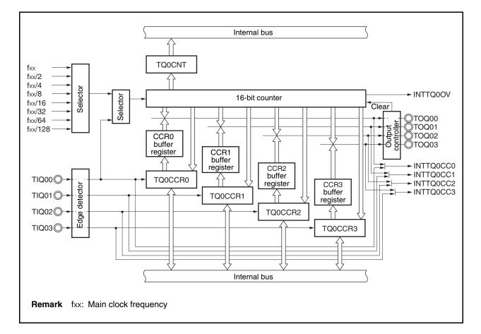
Figure 8-1. Block Diagram of TMQ0
