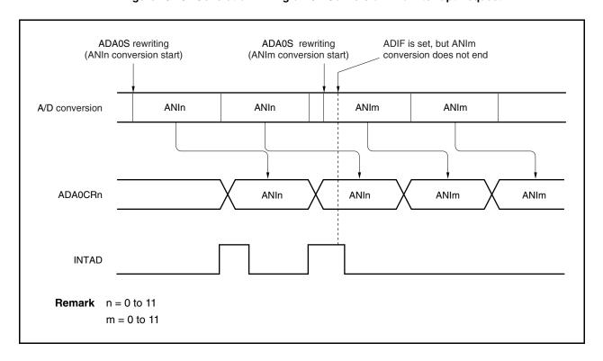
Figure 13-13. Generation Timing of A/D Conversion End Interrupt Request
