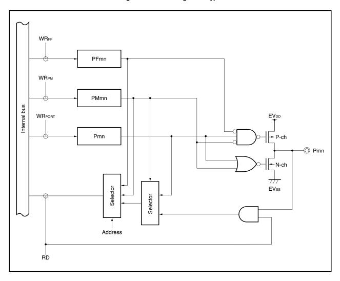
Figure 4-5. Block Diagram of Type C-1
