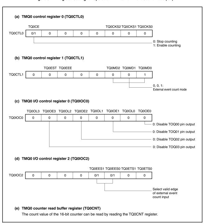
Figure 8-11. Register Setting for Operation in External Event Count Mode (2/2)
