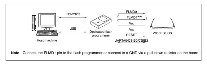
A host machine is required for controlling the dedicated flash programmer.
