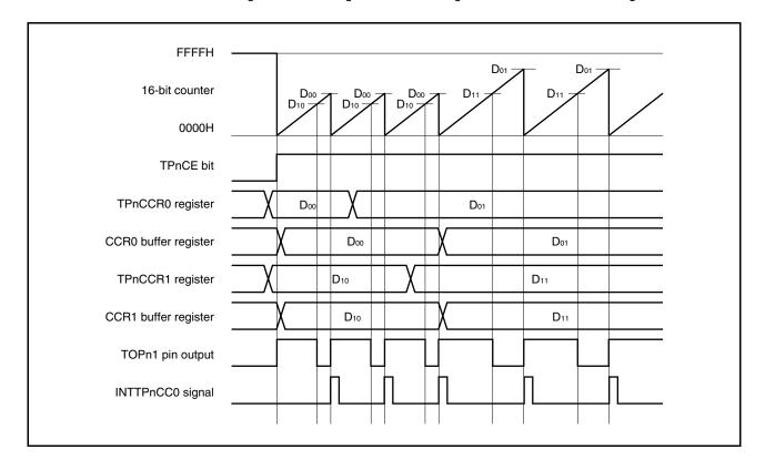
To transfer data from the TPnCCRm register to the CCRm buffer register, the TPnCCR1 register must be written.
