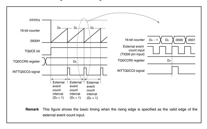
When the TQ0CE bit is set to 1, the value of the 16-bit counter is cleared from FFFFH to 0000H. The counter counts each time the valid edge of external event count input is detected. Additionally, the set value of the TQ0CCR0 register is transferred to the CCR0 buffer register.
