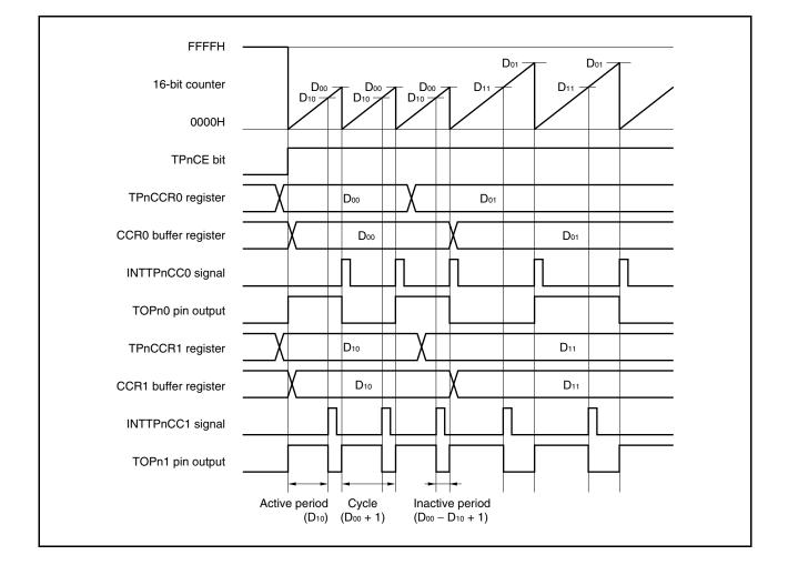
Figure 7-25. Basic Timing in PWM Output Mode
