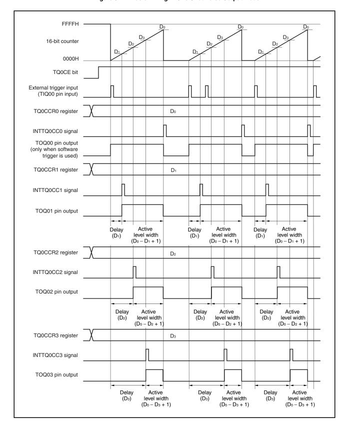
Figure 8-21. Basic Timing in One-Shot Pulse Output Mode
