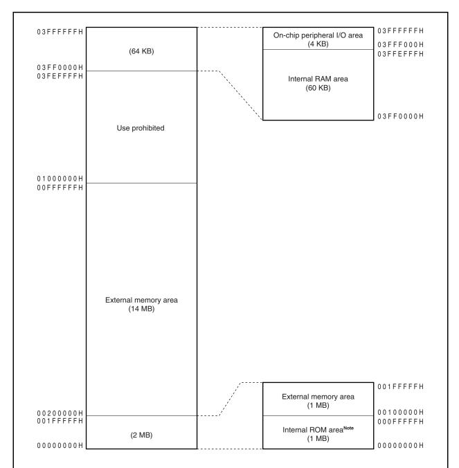
**Note** Fetch access and read access to addresses 00000000H to 000FFFFFH is made to the internal ROM area. However, data write access to these addresses is made to the external memory area.
