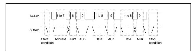
Figure 17-7. I<sup>2</sup>C Bus Serial Data Transfer Timing
