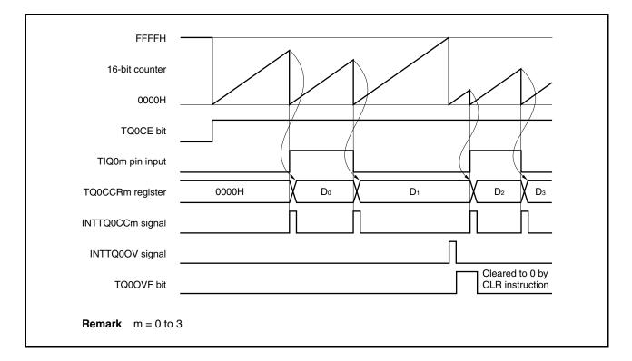
Figure 8-35. Basic Timing in Pulse Width Measurement Mode
