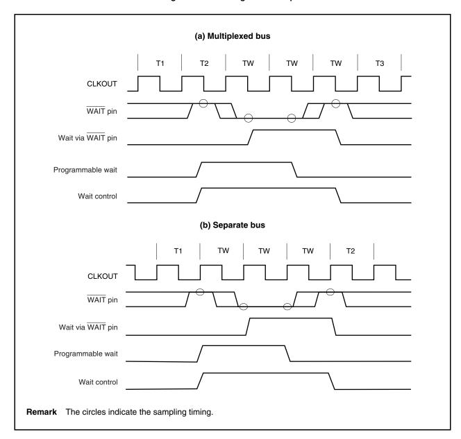
Figure 5-3. Inserting Wait Example
