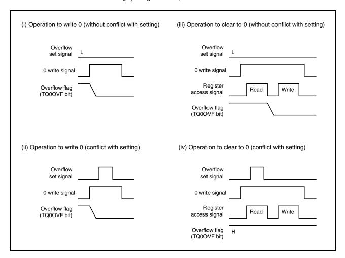
To clear the overflow flag to 0, read the overflow flag to check if it is set to 1, and clear it with the CLR instruction. If 0 is written to the overflow flag without checking if the flag is 1, the set information of overflow may be erased by writing 0 ((ii) in the above chart). Therefore, software may judge that no overflow has occurred even when an overflow actually has occurred.
