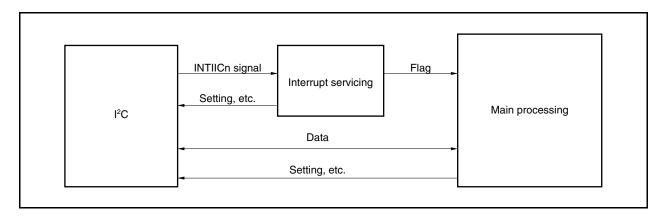
Figure 17-20. Software Outline During Slave Operation
