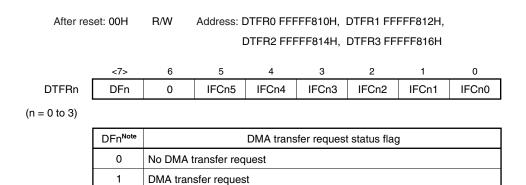
**Note** Do not set the DFn bit to 1 by software. Write 0 to this bit to clear a DMA transfer request if an interrupt that is specified as the cause of starting DMA transfer occurs while DMA transfer is disabled.
