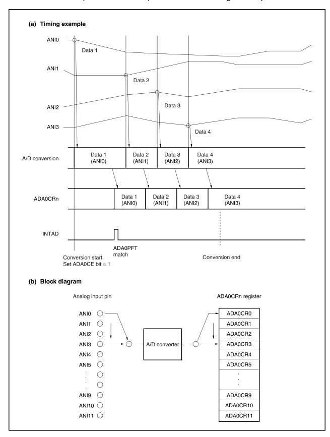
Figure 13-11. Timing Example of One-Shot Scan Mode Operation (When Power-Fail Comparison Is Made: ADAOS Register = 03H)
