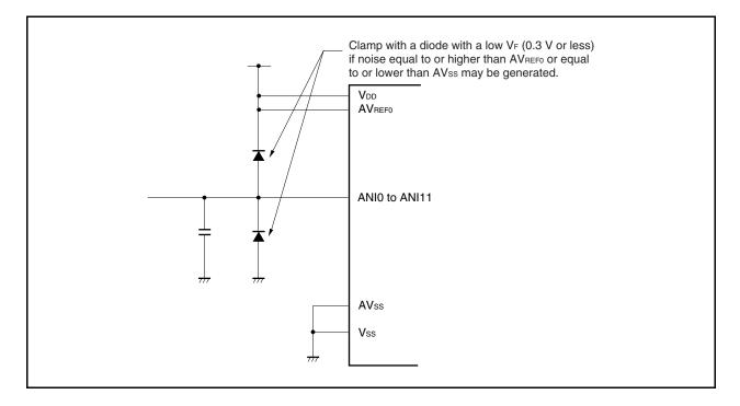
Figure 13-12. Processing of Analog Input Pin
