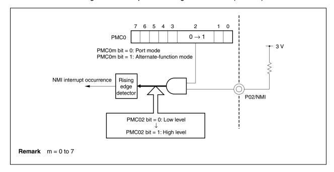
Figure 4-33. Example of Switching from P02 to NMI (Incorrect)
