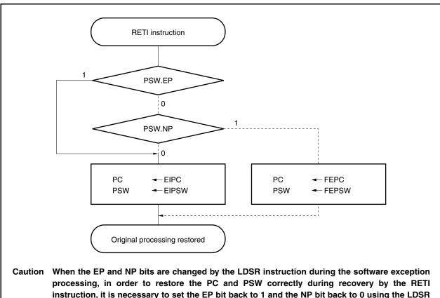
instruction, it is necessary to set the EP bit back to 1 and the NP bit back to 0 using the LDSR instruction immediately before the RETI instruction.
