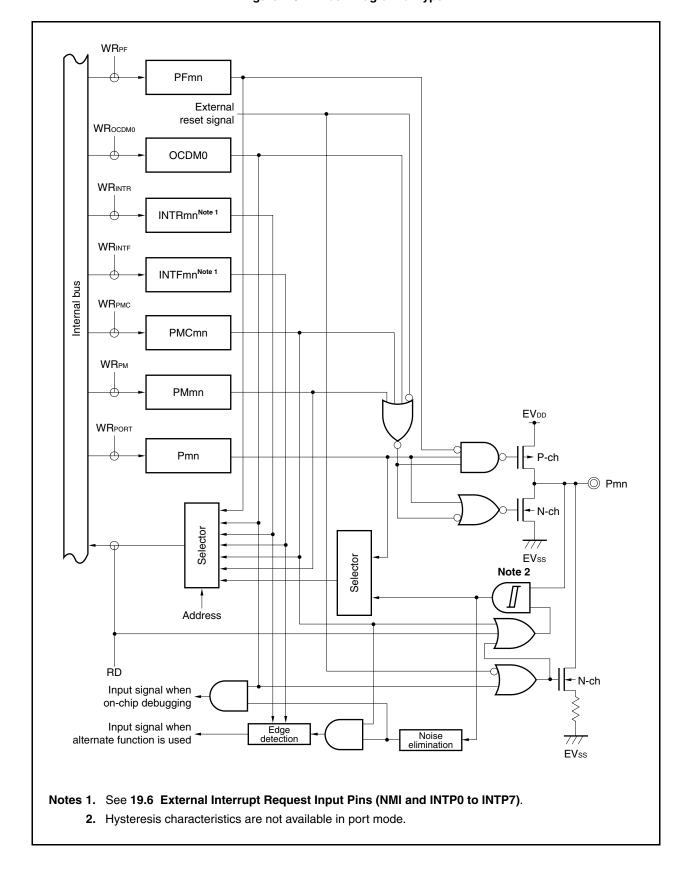
Figure 4-32. Block Diagram of Type AA-1
