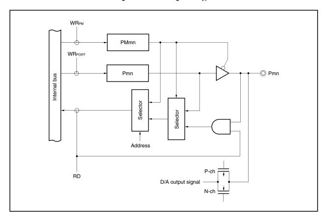
Figure 4-4. Block Diagram of Type A-2
