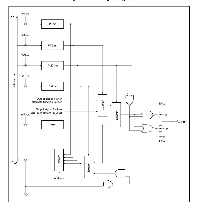
Figure 4-12. Block Diagram of Type G-3
