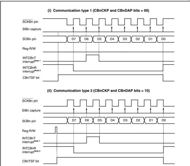
Notes 1. The INTCBnT interrupt is set when the data written to the CBnTX register is transferred to the data shift register in the continuous transmission or continuous transmission/reception mode. In the single transmission or single transmission/reception mode, the INTCBnT interrupt request signal is not generated, but the INTCBnR interrupt request signal is generated upon end of communication.
