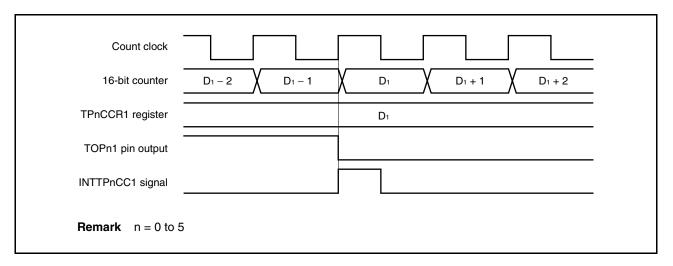
Usually, the INTTPnCC1 signal is generated in synchronization with the next counting up after the count value of the 16-bit counter matches the value of the TPnCCR1 register.
