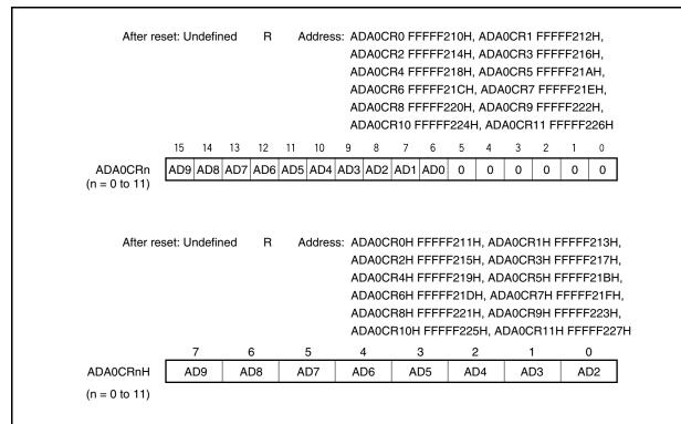
Caution A write operation to the ADA0M0 and ADA0S registers may cause the contents of the ADA0CRn register to become undefined. After the conversion, read the conversion result before writing to the ADA0M0 and ADA0S registers. Correct conversion results may not be read if a sequence other than the above is used.
