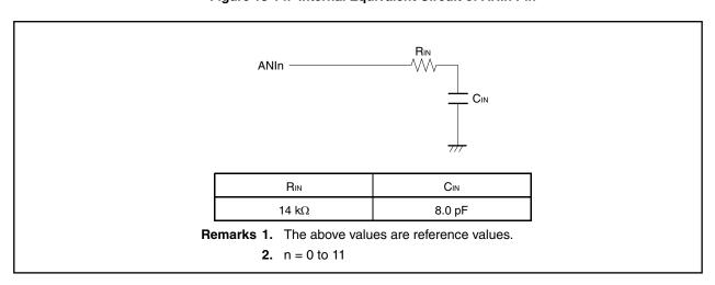
Figure 13-14. Internal Equivalent Circuit of ANIn Pin
