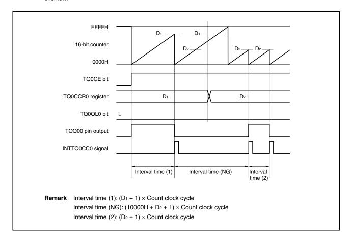
If the value of the TQ0CCR0 register is changed from  $D_1$  to  $D_2$  while the count value is greater than  $D_2$  but less than  $D_1$ , the count value is transferred to the CCR0 buffer register as soon as the TQ0CCR0 register has been rewritten. Consequently, the value of the 16-bit counter that is compared is  $D_2$ .
