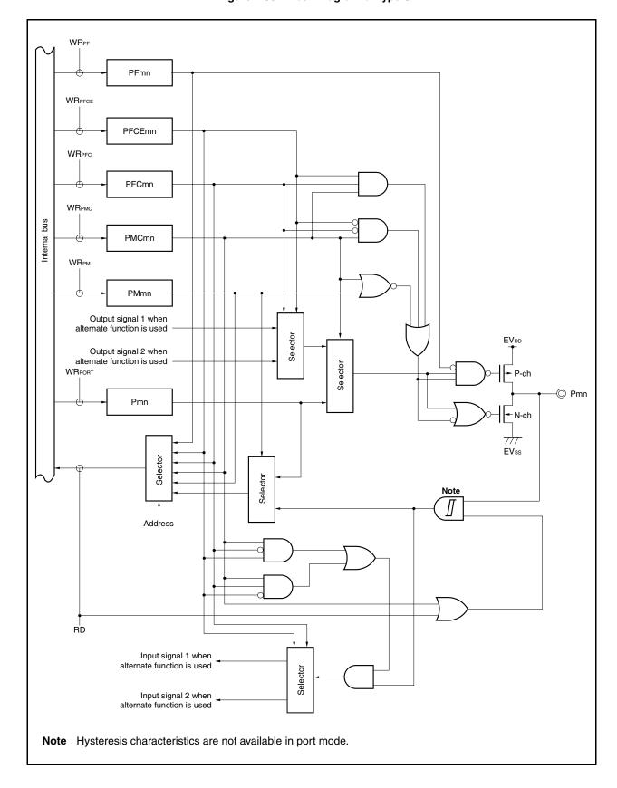
Figure 4-30. Block Diagram of Type U-14
