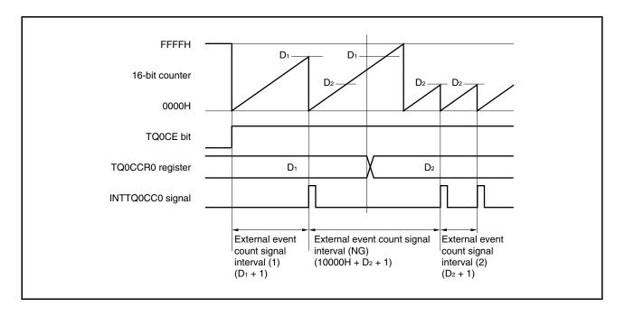
If the value of the TQ0CCR0 register is changed from  $D_1$  to  $D_2$  while the count value is greater than  $D_2$  but less than  $D_1$ , the count value is transferred to the CCR0 buffer register as soon as the TQ0CCR0 register has been rewritten. Consequently, the value that is compared with the 16-bit counter is  $D_2$ .
