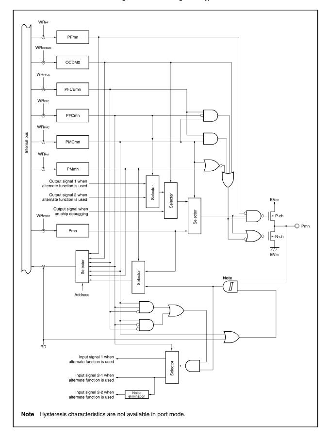
Figure 4-23. Block Diagram of Type U-7
