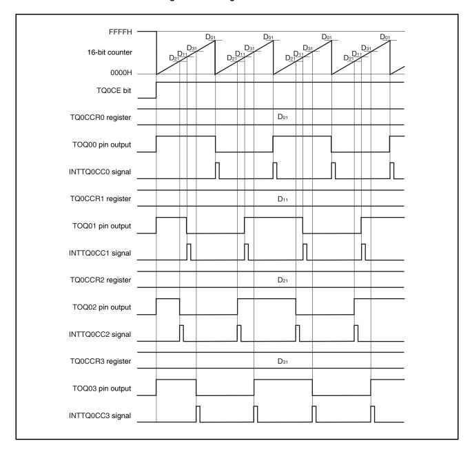
If the set value of the TQ0CCRk register is greater than the set value of the TQ0CCR0 register, the count value of the 16-bit counter does not match the value of the TQ0CCRk register. Consequently, the INTTQ0CCk signal is not generated, nor is the output of the TQQ0k pin changed.
