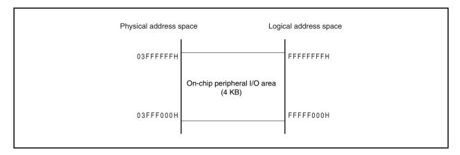
Peripheral I/O registers that have functions to specify the operation mode for and monitor the status of the on-chip peripheral I/O are mapped to the on-chip peripheral I/O area. Program cannot be fetched from this area.
