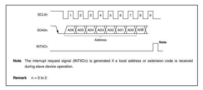
The slave address and the eighth bit, which specifies the transfer direction as described in 17.6.3 Transfer direction specification below, are written together to IIC shift register n (IICn) and then output. Received addresses are written to the IICn register (n = 0 to 2).
