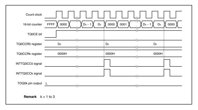
To output a 100% waveform, set a value of (set value of TQ0CCR0 register + 1) to the TQ0CCRk register. If the set value of the TQ0CCR0 register is FFFFH, 100% output cannot be produced.
