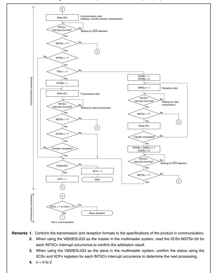
Figure 17-19. Master Operation in Multimaster System (3/3)
