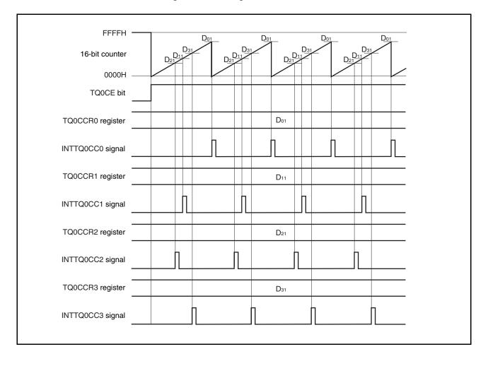
If the set value of the TQ0CCRk register is greater than the set value of the TQ0CCR0 register, the INTTQ0CCk signal is not generated because the count value of the 16-bit counter and the value of the TQ0CCRk register do not match.
