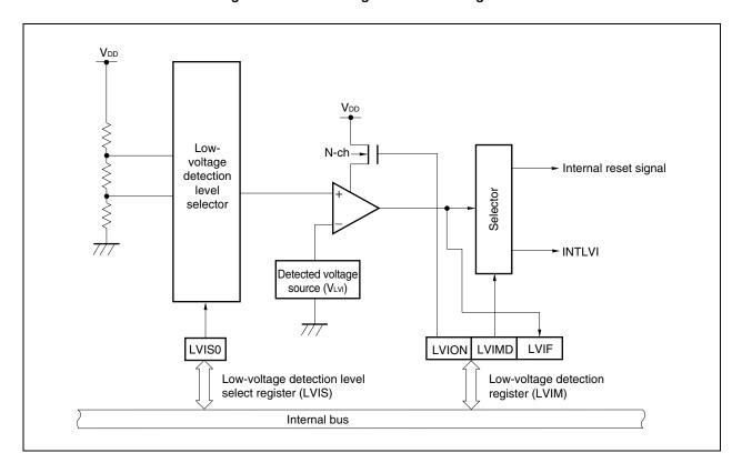
Figure 24-1. Block Diagram of Low-Voltage Detector
