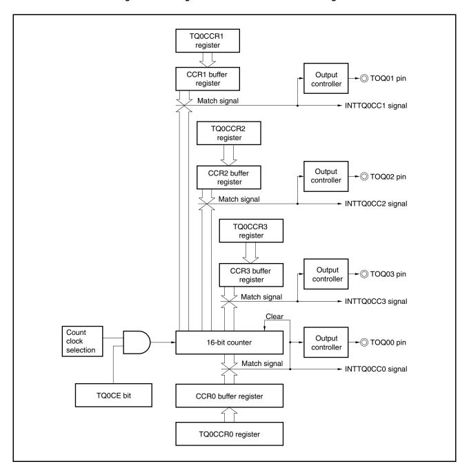
If the set value of the TQ0CCRk register is less than the set value of the TQ0CCR0 register, the INTTQ0CCk signal is generated once per cycle. At the same time, the output of the TOPQ0k pin is inverted. The TOQ0k pin outputs a square wave with the same cycle as that output by the TOQ00 pin.
