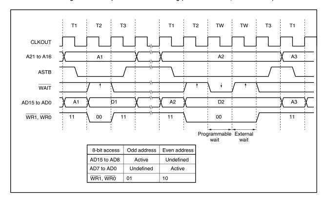
Figure 5-6. Multiplexed Bus Write Timing (Bus Size: 16 Bits, 16-Bit Access)
