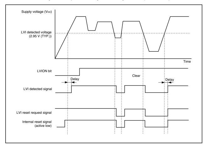
Figure 24-2. Operation Timing of Low-Voltage Detector (LVIMD Bit = 1)
