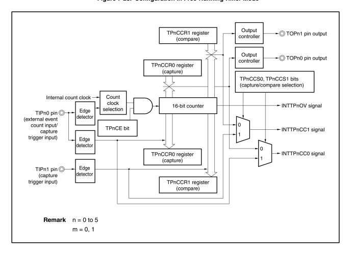
Figure 7-28. Configuration in Free-Running Timer Mode
