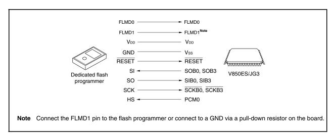
The dedicated flash programmer outputs the transfer clock, and the V850ES/JG3 operates as a slave.
