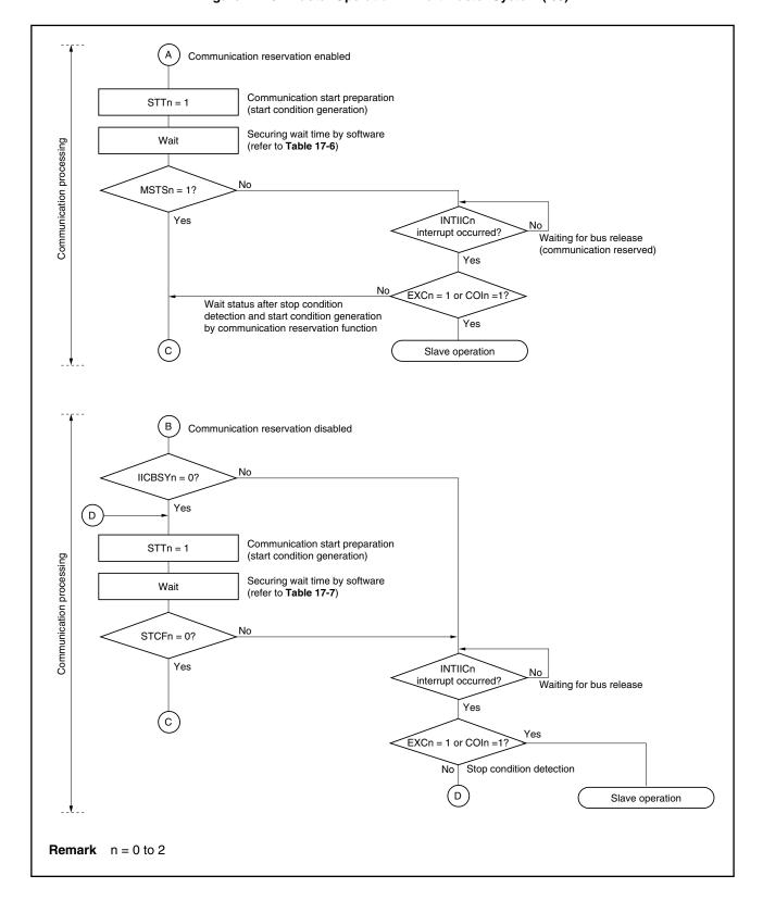
Figure 17-19. Master Operation in Multimaster System (2/3)
