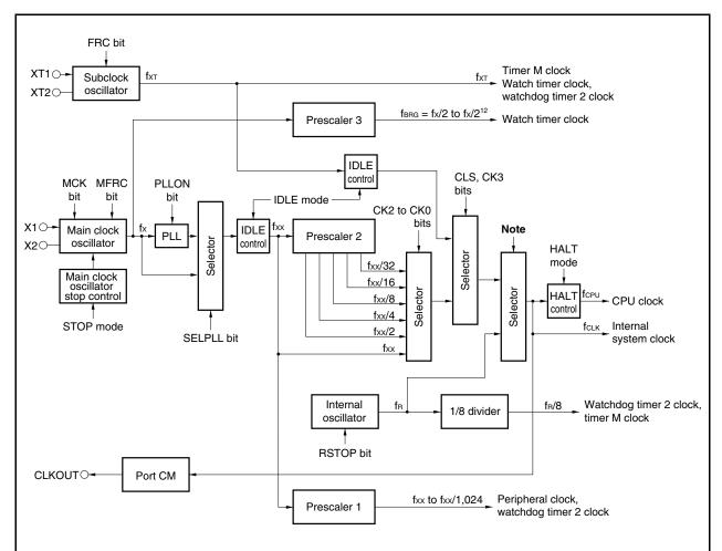
**Note** The internal oscillation clock is selected when watchdog timer 2 overflows during the oscillation stabilization time.
