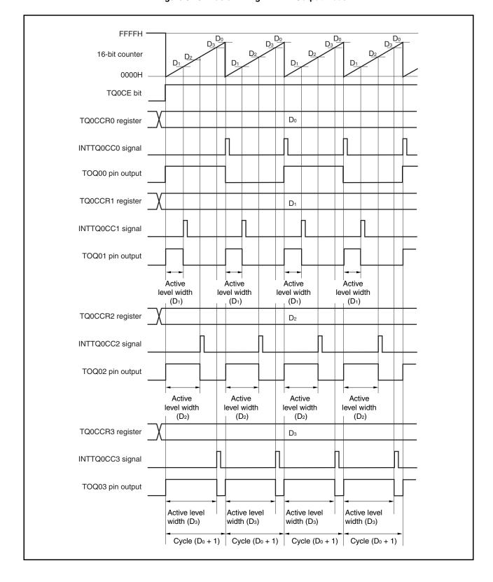
Figure 8-25. Basic Timing in PWM Output Mode
