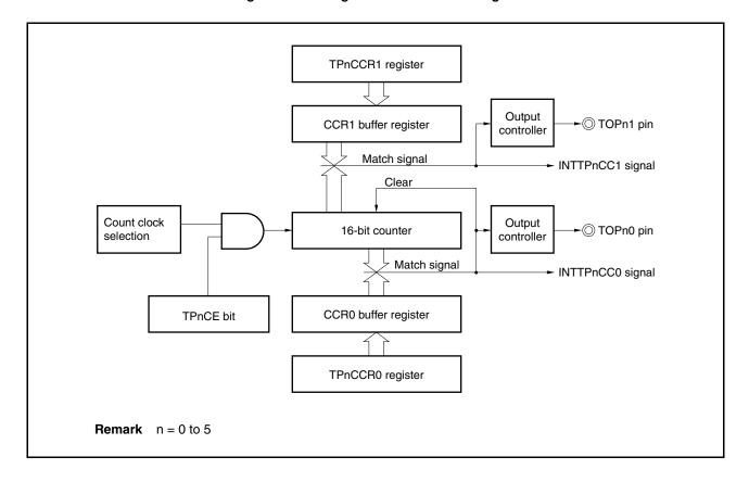
If the set value of the TPnCCR1 register is less than the set value of the TPnCCR0 register, the INTTPnCC1 signal is generated once per cycle. At the same time, the output of the TOPn1 pin is inverted. The TOPn1 pin outputs a square wave with the same cycle as that output by the TOPn0 pin.
