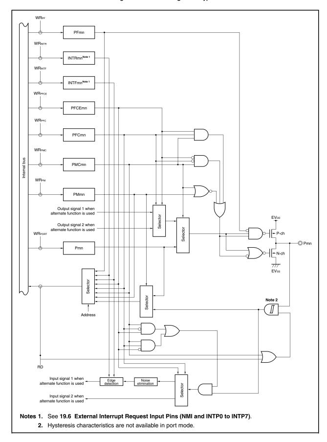
Figure 4-31. Block Diagram of Type U-15
