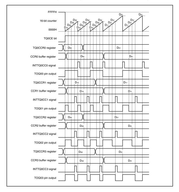
To transfer data from the TQ0CCRm register to the CCRm buffer register, the TQ0CCR1 register must be written.
