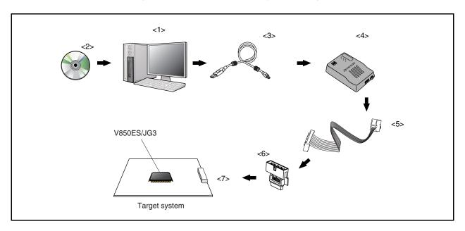
Figure A-3. On-Chip Emulation System Configuration
