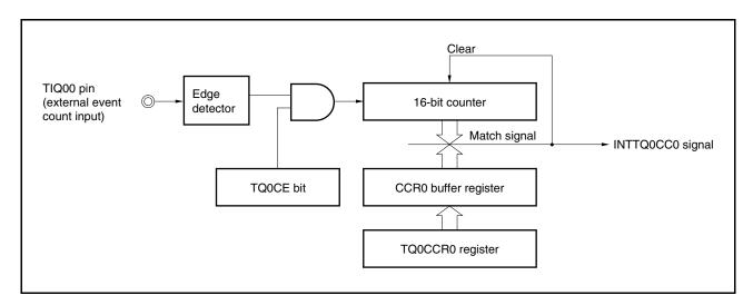
Figure 8-9. Configuration in External Event Count Mode
