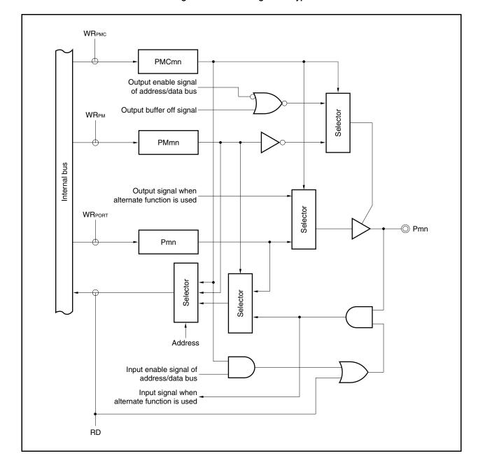
Figure 4-8. Block Diagram of Type D-3
