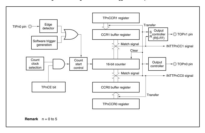
Figure 7-16. Configuration in External Trigger Pulse Output Mode
