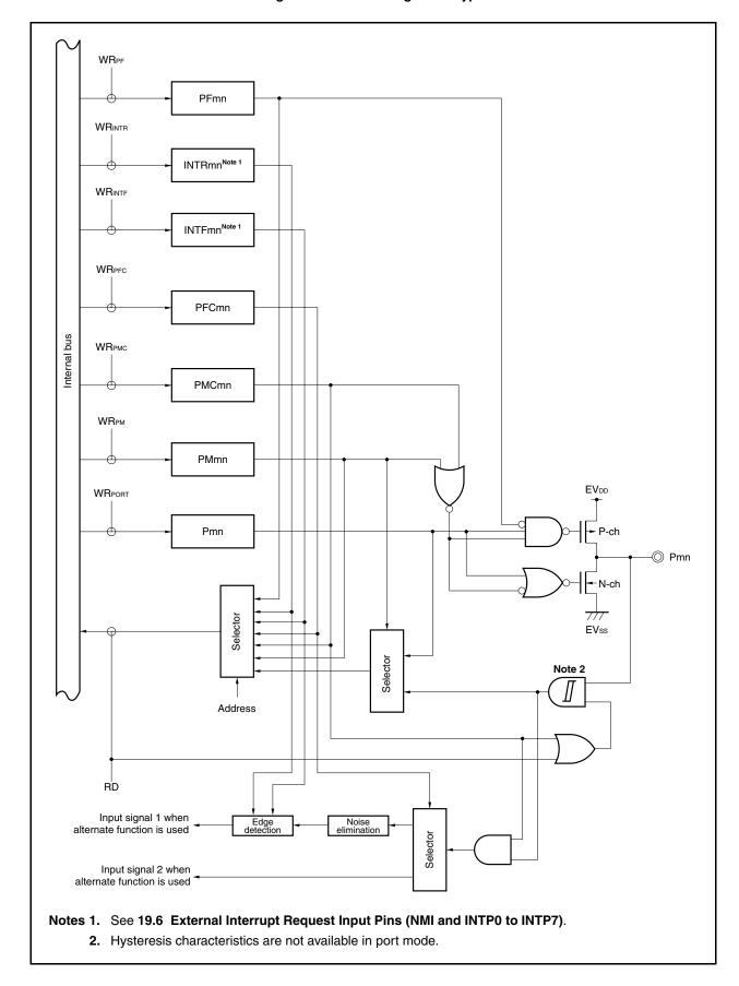
Figure 4-17. Block Diagram of Type N-1
