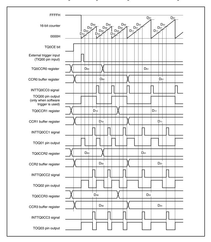
In order to transfer data from the TQ0CCRm register to the CCRm buffer register, the TQ0CCR1 register must be written.
