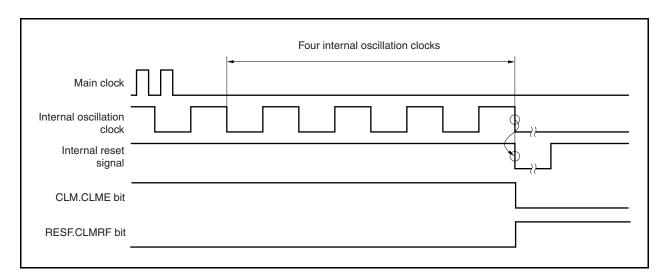
Figure 23-2. Reset Period Due to That Oscillation of Main Clock Is Stopped
