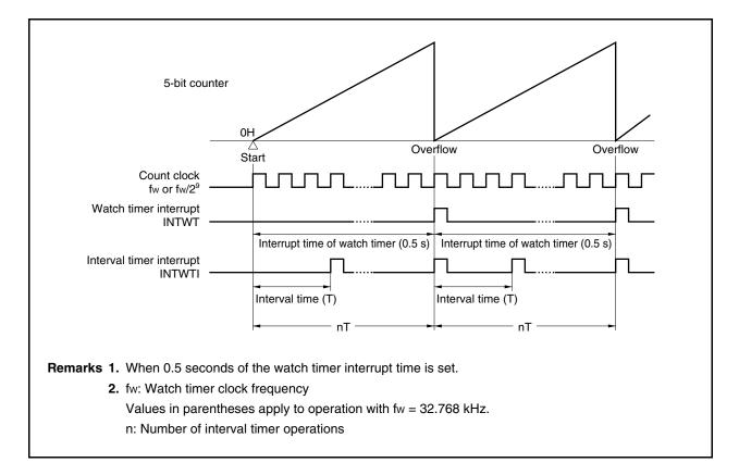
Figure 10-2. Operation Timing of Watch Timer/Interval Timer
