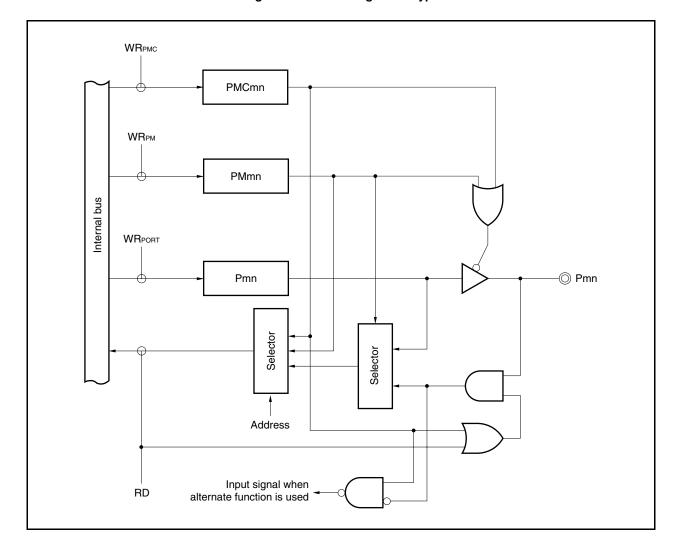
Figure 4-6. Block Diagram of Type D-1
