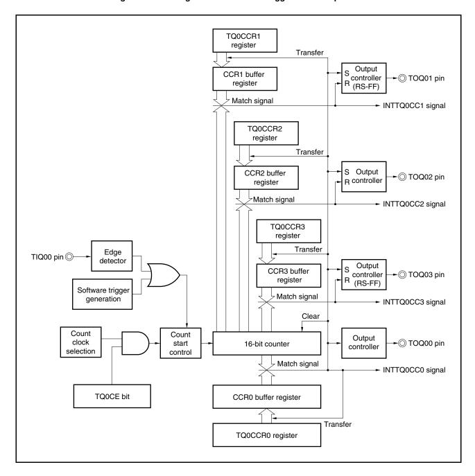
Figure 8-16. Configuration in External Trigger Pulse Output Mode
