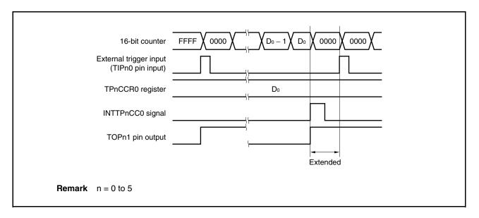
If the trigger is detected immediately before the INTTPnCC0 signal is generated, the INTTPnCC0 signal is not generated. The 16-bit counter is cleared to 0000H, the TOPn1 pin is asserted, and the counter continues counting. Consequently, the inactive period of the PWM waveform is shortened.
