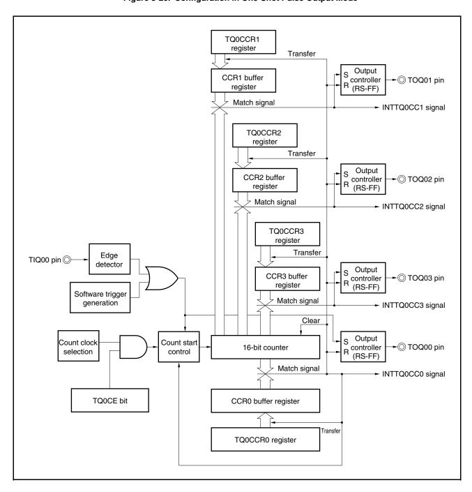
Figure 8-20. Configuration in One-Shot Pulse Output Mode
