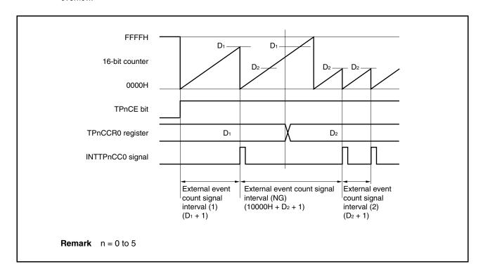
If the value of the TPnCCR0 register is changed from D1 to D2 while the count value is greater than D2 but less than D1, the count value is transferred to the CCR0 buffer register as soon as the TPnCCR0 register has been rewritten. Consequently, the value that is compared with the 16-bit counter is D2.
