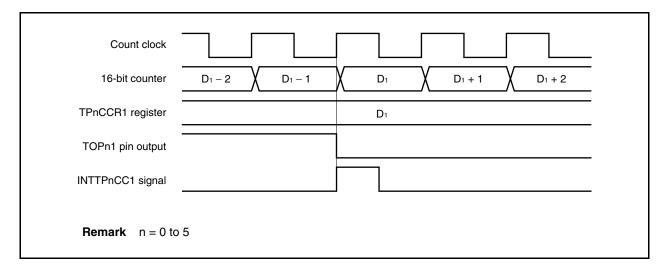
Usually, the INTTPnCC1 signal is generated in synchronization with the next count up, after the count value of the 16-bit counter matches the value of the TPnCCR1 register.
