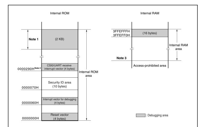
Figure 28-4. Memory Spaces Where Debug Monitor Programs Are Allocated
