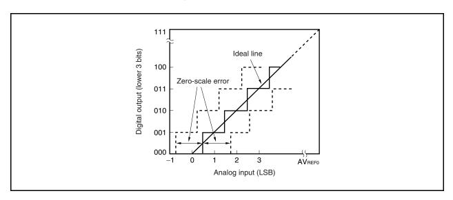
Figure 13-18. Zero-Scale Error
