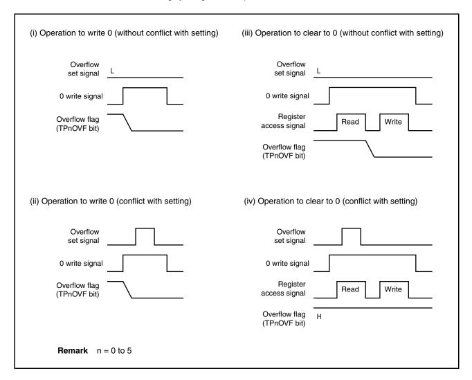
To clear the overflow flag to 0, read the overflow flag to check if it is set to 1, and clear it with the CLR instruction. If 0 is written to the overflow flag without checking if the flag is 1, the set information of overflow may be erased by writing 0 ((ii) in the above chart). Therefore, software may judge that no overflow has occurred even when an overflow actually has occurred.
