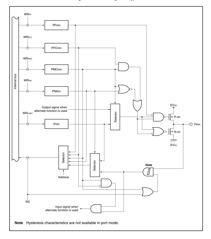
Figure 4-10. Block Diagram of Type G-1
