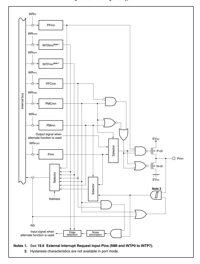
Figure 4-18. Block Diagram of Type N-2
