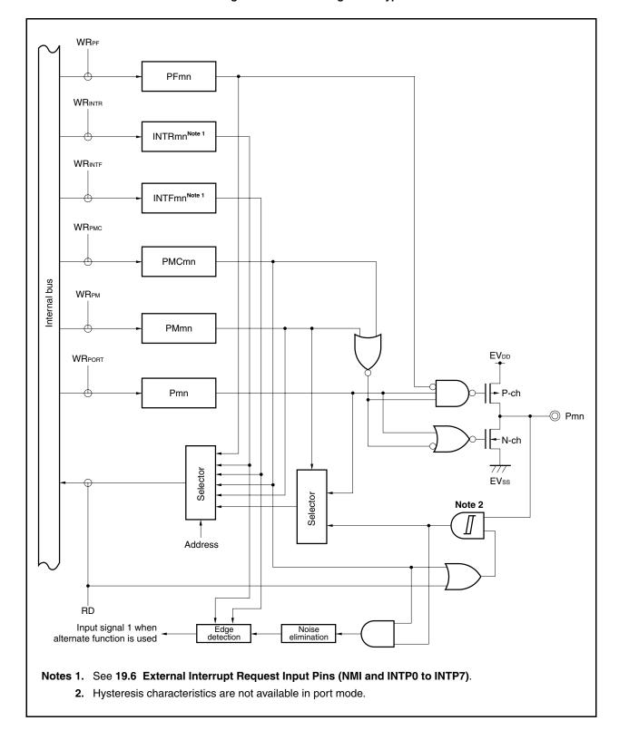
Figure 4-16. Block Diagram of Type L-1
