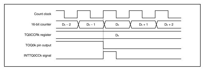
Usually, the INTTQ0CCk signal is generated when the 16-bit counter counts up next time after its count value matches the value of the TQ0CCRk register.
