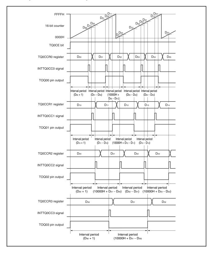
When performing an interval operation in the free-running timer mode, two intervals can be set with one channel.
